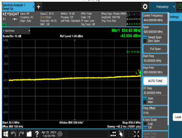
Plot 8-521. Conducted Spurious Emission Plot 30 MHz to 858 MHz
