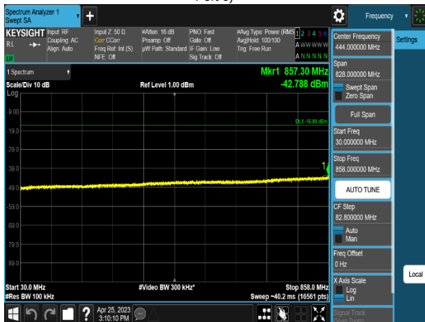
Plot 8-533. Conducted Spurious Emission Plot 30 MHz to 858 MHz (MSR 2NC_NR n5_1C_5M+LTE B5_1C_5M_2T_QPSK-Mid Channel, Port 0)
