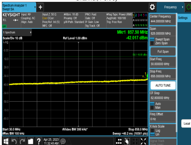
Plot 8-509. Conducted Spurious Emission Plot 30 MHz to 858 MHz (MSR 3C_DSS B(n)5_2C_10M+10M+LTE B5_1C_5M_2T_QPSK-Mid Channel, Port 0)
