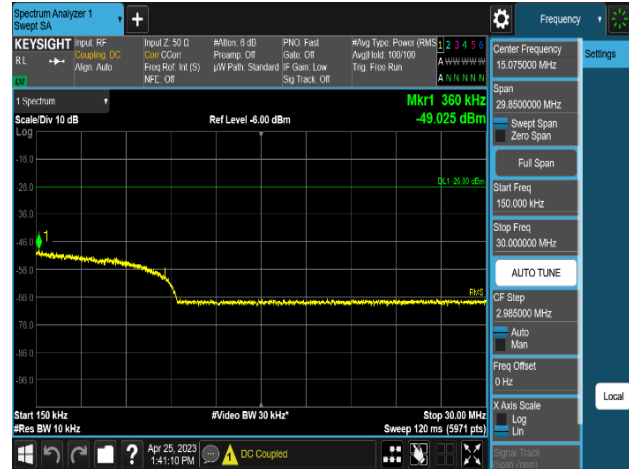
Plot 8-520. Conducted Spurious Emission Plot 150 kHz to 30 MHz
