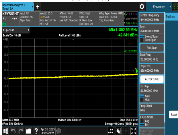
Plot 8-527. Conducted Spurious Emission Plot 30 MHz to 858 MHz (MSR 3C_NR n5_2C_10M+10M+LTE B5_1C_5M_2T_QPSK-Mid Channel, Port 0)
