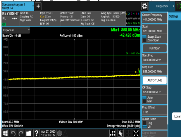
Plot 8-654. Conducted Spurious Emission Plot 30 MHz to 858 MHz
