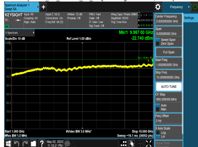
Plot 8-681. Conducted Spurious Emission Plot 1 GHz to 10 GHz (NR n5_2C_5M+5M_4T_16QAM - High Channel, Port 0)
