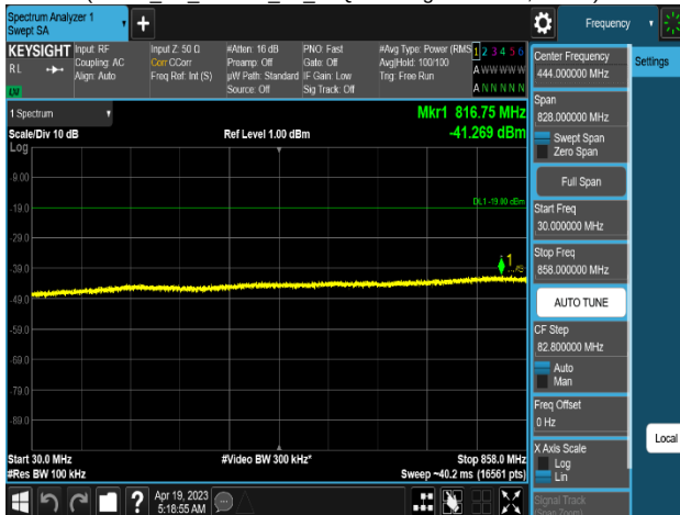
Plot 8-678. Conducted Spurious Emission Plot 30 MHz to 858 MHz (NR n5_2C_5M+5M_4T_16QAM - High Channel, Port 0)
