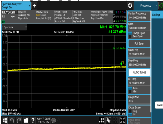
Plot 8-666. Conducted Spurious Emission Plot 30 MHz to 858 MHz (NR_n5_1C_10M_4T_64QAM - Middle Channel, Port 0)
