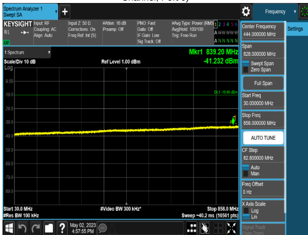
Plot 8-732. Conducted Spurious Emission Plot 30 MHz to 858 MHz (MSR 2C_DSS B(n)5_1C_10M+NR n5_1C_5M_4T_QPSK - Low Channel, Port 0)
