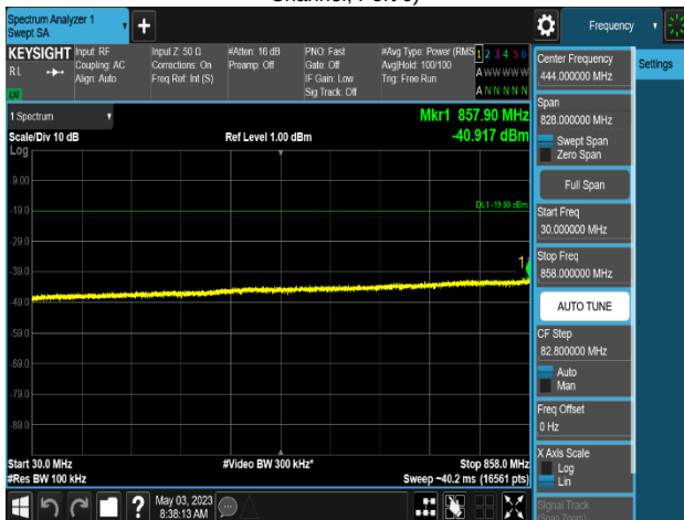
Plot 8-744. Conducted Spurious Emission Plot 30 MHz to 858 MHz (MSR 2NC_DSS B(n)5_1C_10M+NR n5_1C_5M_4T_QPSK - Middle Channel, Port 0)
