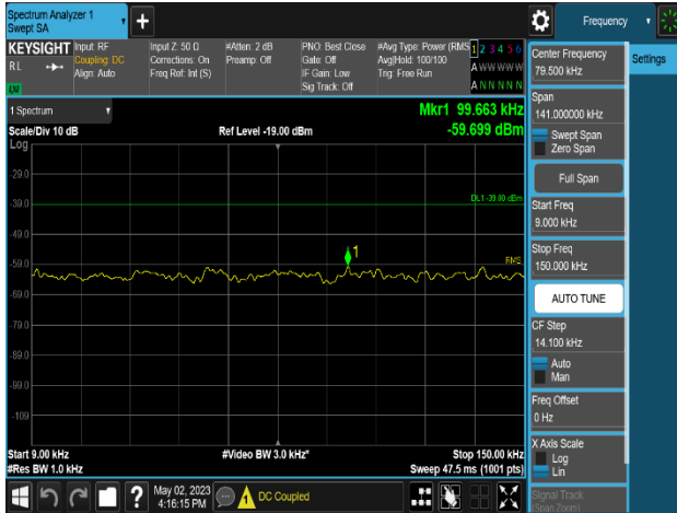
Plot 8-736. Conducted Spurious Emission Plot 9 kHz to 150 kHz (MSR 2C_DSS B(n)5_1C_10M+NR n5_1C_15M_4T_16QAM - Middle Channel, Port 0)
