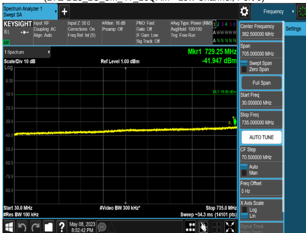
Plot 8-768. Conducted Spurious Emission Plot 30 MHz to 735 MHz (LTE B13_1C_5M_4T_16QAM - Low Channel, Port 0)
