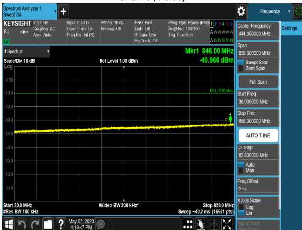
Plot 8-738. Conducted Spurious Emission Plot 30 MHz to 858 MHz (MSR 2C_DSS B(n)5_1C_10M+NR n5_1C_15M_4T_16QAM - Middle Channel, Port 0)
