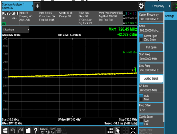
Plot 8-780. Conducted Spurious Emission Plot 30 MHz to 735 MHz (LTE B13_2C_5M+5M_4T_QPSK - Middle Channel, Port 0)
