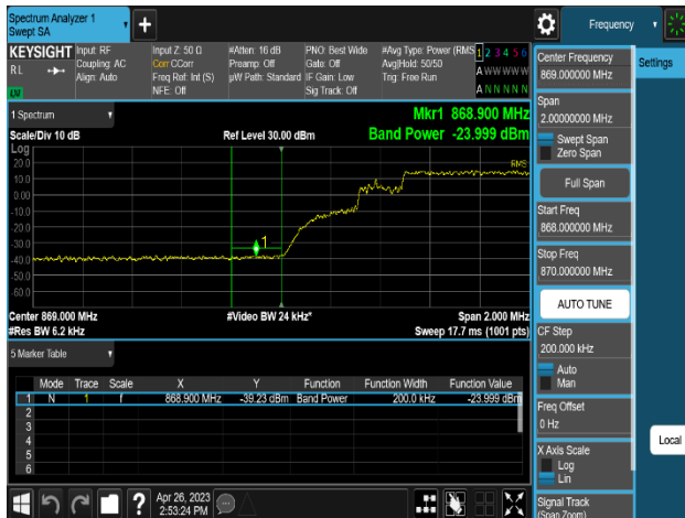
Plot 8-337. Band Edge Emission Summary Data Plot (MSR 3C_DSS B(n)5_1C_10M+NR n5_1C_5M+LTE B5_1C_5M_QPSK - Low Channel 2T, Port 1)
