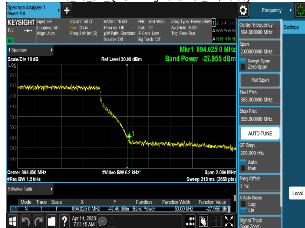
Plot 8-358. Band Edge Emission Summary Data Plot (LTE B5_1C_5M_256QAM - High Channel 4T, Port 1)
