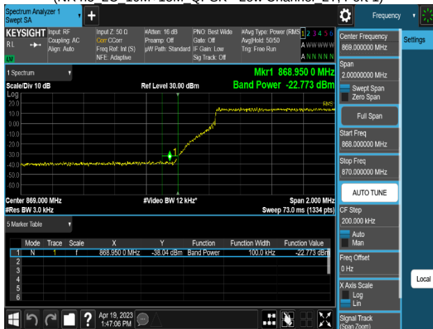
Plot 8-317. Band Edge Emission Summary Data Plot (NR n5_2NC_10M+15M_QPSK - Low Channel_2T, Port 1)
