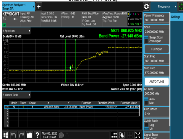
Plot 8-401. Band Edge Emission Summary Data Plot (MSR 2NC_DSS B(n)5_1C_10M+NR n5_1C_5M_QPSK - Low Channel 4T, Port 1)
