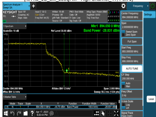
Plot 8-376. Band Edge Emission Summary Data Plot (NR n5_1C_10M_256QAM - High Channel_4T, Port 1)
