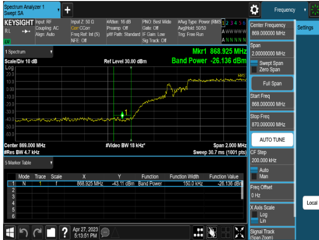
Plot 8-385. Band Edge Emission Summary Data Plot (MSR 2C_DSS B(n)5_1C_10M+LTE B5_1C_5M_16QAM - Low Channel 4T, Port 2)
