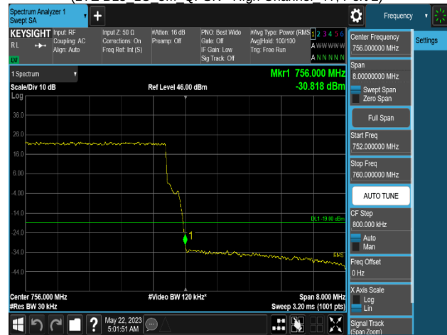
Plot 8-412. Band Edge Emission Summary Data Plot (LTE B13 1C 10M QPSK - High Channel 4T, Port 1)
