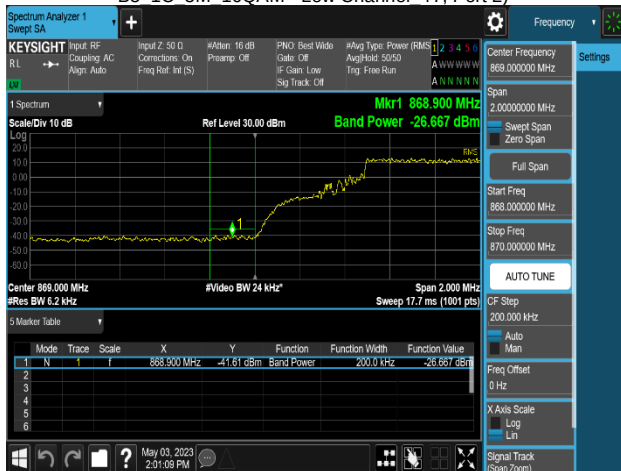
Plot 8-407. Band Edge Emission Summary Data Plot (MSR 3NC_DSS B(n)5_1C_10M+NR n5_1C_5M+LTE B5_1C_5M_QPSK - Low Channel 4T, Port 1)
