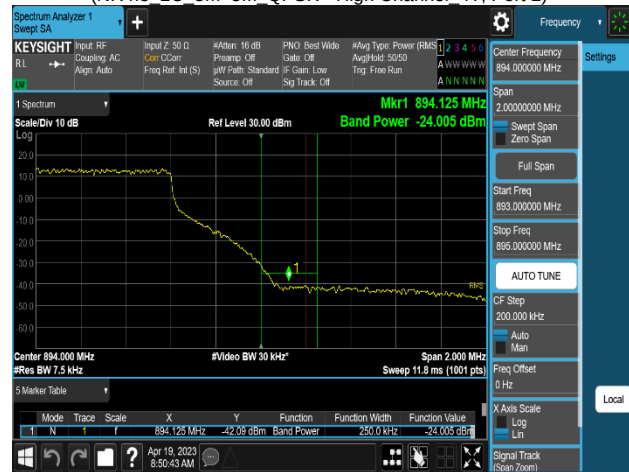
Plot 8-382. Band Edge Emission Summary Data Plot (NR n5_2C_10M+15M_16QAM - High Channel 4T, Port 2)
