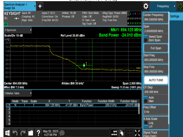
Plot 8-400. Band Edge Emission Summary Data Plot (MSR 2C_DSS B(n)5_1C_10M+NR n5_1C_15M_16QAM - High Channel 4T, Port 1)
