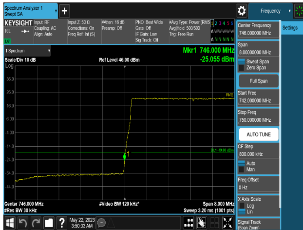
Plot 8-421. Band Edge Emission Summary Data Plot (Multi-Band_LTE B13_2C_5M+5M+DSS B(n)5_1C_10M+NR n5_1C_10M+LTE B5_1C_5M_QPSK – Low Channel _4T, Port 3)
