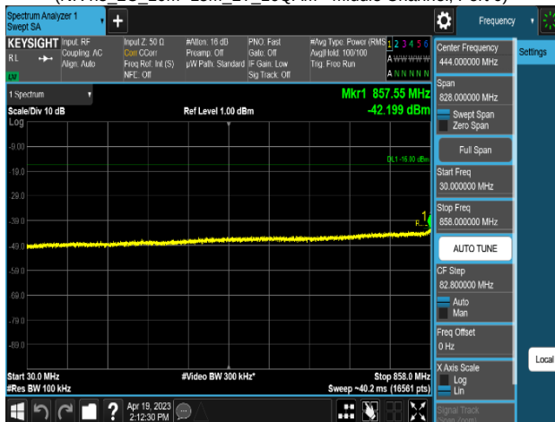
Plot 8-491. Conducted Spurious Emission Plot 30 MHz to 858 MHz (NR n5_2C_10M+15M_2T_16QAM - Middle Channel, Port 0)
