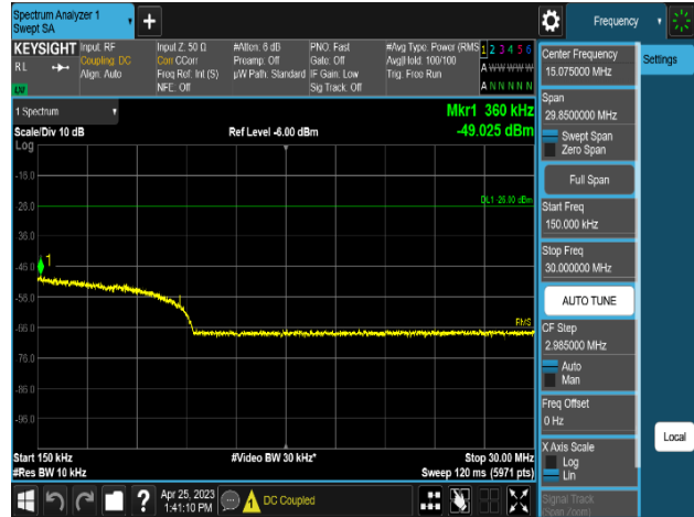
Plot 8-520. Conducted Spurious Emission Plot 150 kHz to 30 MHz (MSR 2C_NR n5_1C_5M+LTE B5_1C_5M_2T_16QAM-Middle Channel, Port 0)
