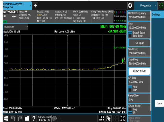
Plot 8-522. Conducted Spurious Emission Plot 858 MHz to 868 MHz (MSR 2C_NR n5_1C_5M+LTE B5_1C_5M_2T_16QAM-Middle Channel, Port 0)
