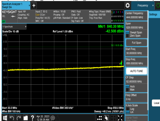
Plot 8-455. Conducted Spurious Emission Plot 30 MHz to 858 MHz (DSS B(n)5_1C_10M(5:5 Ratio)_2T_256QAM - Low Channel, Port 1)
