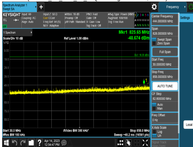
Plot 8-431. Conducted Spurious Emission Plot 30 MHz to 858 MHz (LTE B5_1C_10M_2T_16QAM - High Channel, Port 0)
