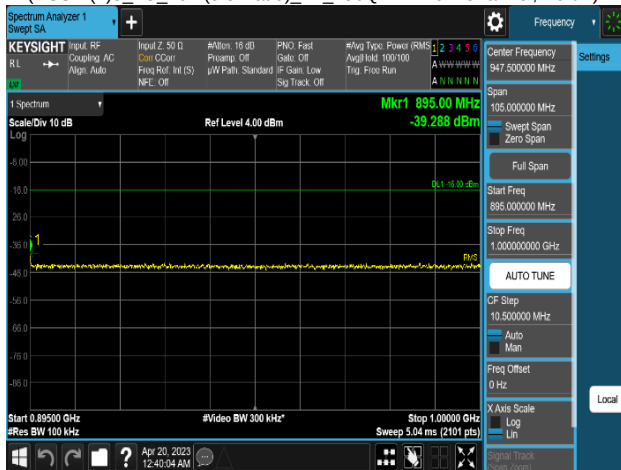
Plot 8-457. Conducted Spurious Emission Plot 895 MHz to 1 GHz (DSS B(n)5_1C_10M(5:5 Ratio)_2T_256QAM - Low Channel, Port 1)
