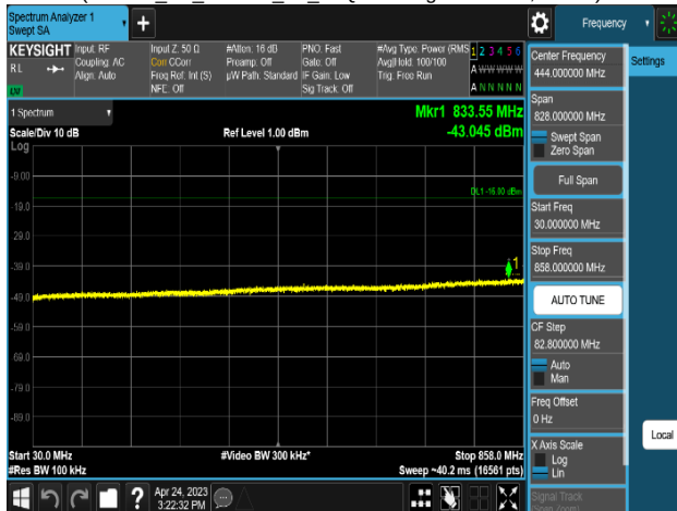
Plot 8-437. Conducted Spurious Emission Plot 30 MHz to 858 MHz (LTE B5_2C_5M+5M_2T_16QAM - High Channel, Port 0)
