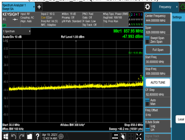
Plot 8-479. Conducted Spurious Emission Plot 30 MHz to 858 MHz (NR n5_1C_15M_2T_64QAM - Low Channel, Port 0)
