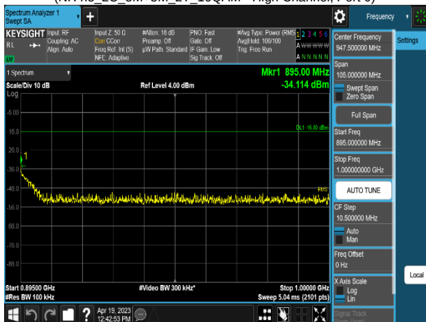
Plot 8-487. Conducted Spurious Emission Plot 895 MHz to 1 GHz (NR n5_2C_5M+5M_2T_16QAM - High Channel, Port 0)
