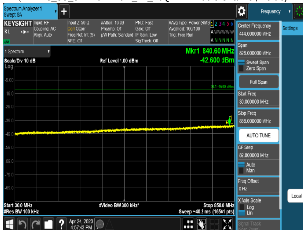
Plot 8-443. Conducted Spurious Emission Plot 30 MHz to 858 MHz (LTE B5_3C_5M+10M+10M_2T_16QAM - Middle Channel, Port 0)
