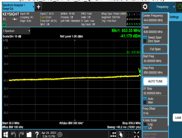
Plot 8-449. Conducted Spurious Emission Plot 30 MHz to 858 MHz
