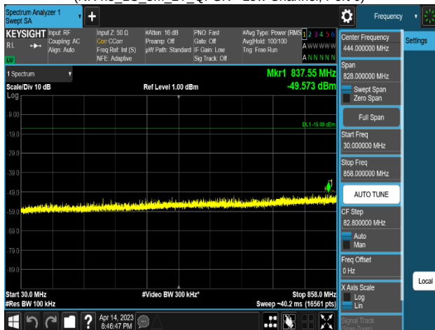
Plot 8-467. Conducted Spurious Emission Plot 30 MHz to 858 MHz (NR n5_1C_5M_2T_QPSK - Low Channel, Port 0)
