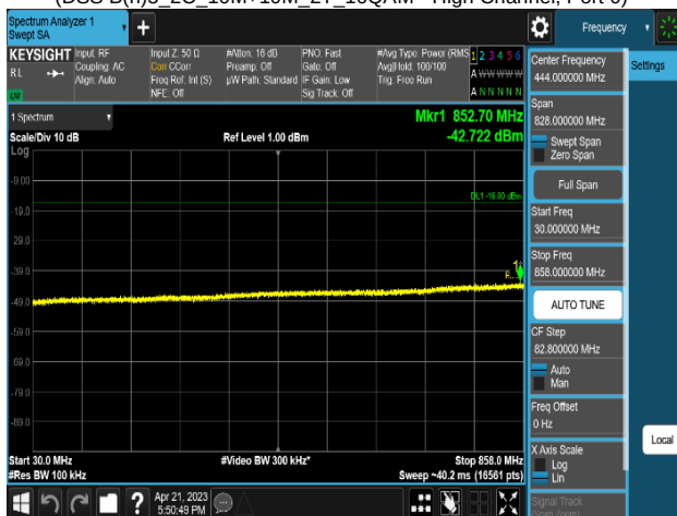
Plot 8-461. Conducted Spurious Emission Plot 30 MHz to 858 MHz
