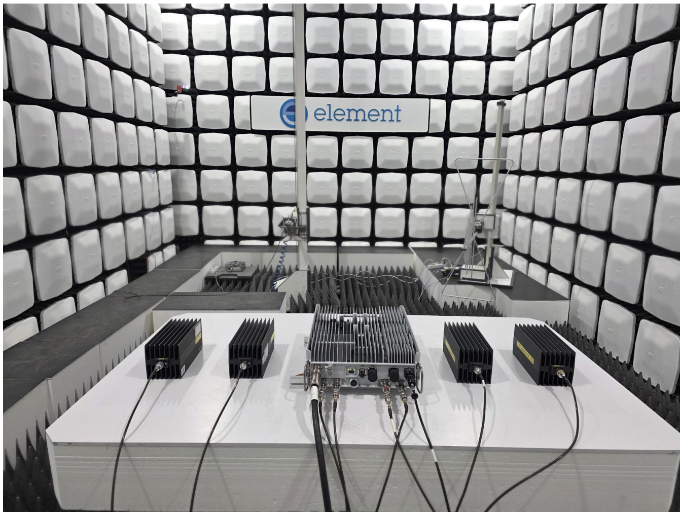
Above 1GHz radiated Test Instrument & Measurement Setup
