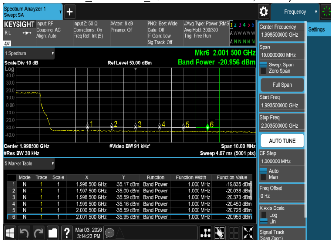
Plot 8-83. Conducted Spurious Emission Plot 1.996 GHz to 2.002 GHz
