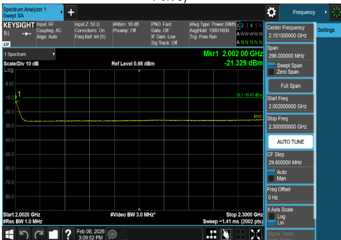
Plot 8-47. Conducted Spurious Emission Plot 2.002 GHz to 2.3 GHz
