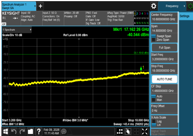
Plot 8-49. Conducted Spurious Emission Plot 3.2 GHz to 18 GHz
