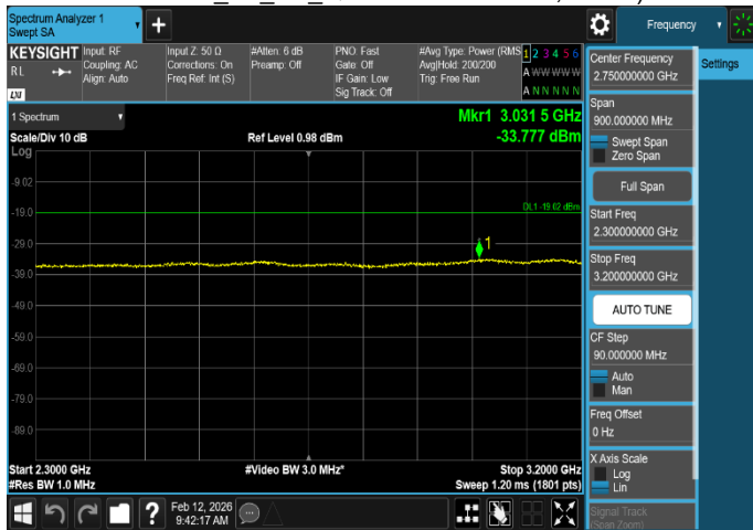
Plot 8-74. Conducted Spurious Emission Plot 2.3 GHz to 3.2GHz (MSR_2NC_B/n66_LTE_10M_NB-IoT Guard band+NR_1C_5M_QPSK - Mid Channel, Port 3)
