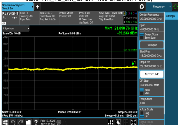
Plot 8-76. Conducted Spurious Emission Plot 18 GHz to 22 GHz (MSR_2NC_B/n66_LTE_10M_NB-IoT Guard band+NR_1C_5M_QPSK - Mid Channel, Port 3)
