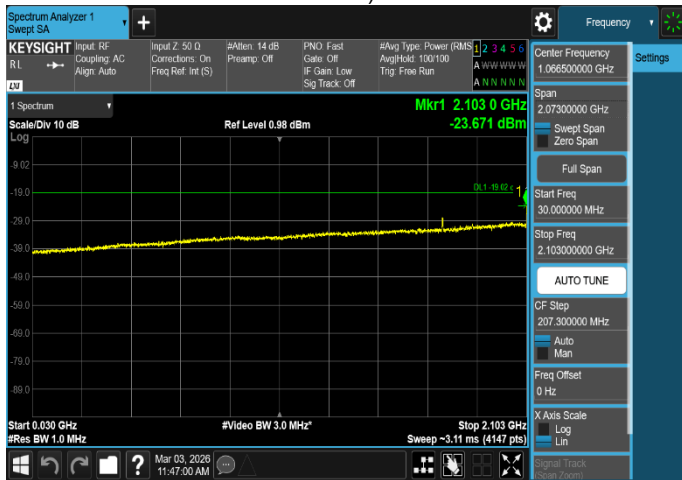
Plot 8-62. Conducted Spurious Emission Plot 30 MHz to 2.103 GHz
