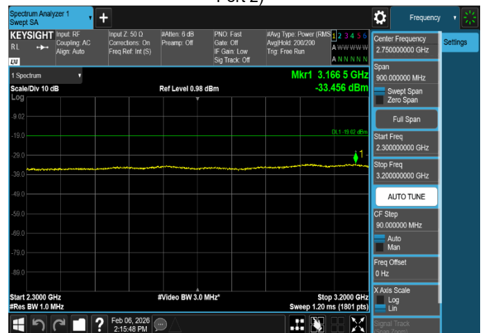
Plot 8-65. Conducted Spurious Emission Plot 2.3 GHz to 3.2 GHz
