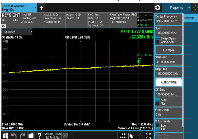
Plot 8-53. Conducted Spurious Emission Plot 30 MHz to 1.923 GHz
