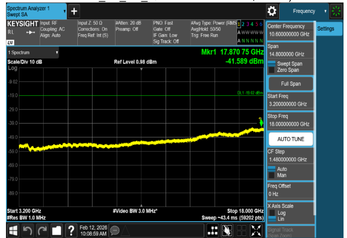
Plot 8-75. Conducted Spurious Emission Plot 3.2 GHz to 18 GHz (MSR_2NC_B/n66_LTE_10M_NB-IoT Guard band+NR_1C_5M_QPSK - Mid Channel, Port 3)
