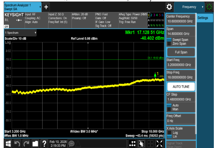
Plot 8-58. Conducted Spurious Emission Plot 3.2 GHz to 18 GHz (LTE_B25_2NC_5M+10M_NB-IoT Guard band_ QPSK - Mid Channel, Port 1)
