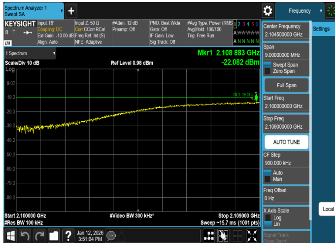
Plot 8-52. Conducted Spurious Emission Plot 2.1 GHz to 2.109 GHz
