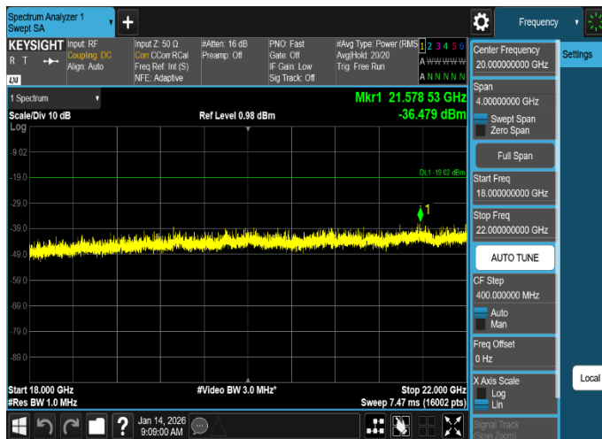
Plot 8-74. Conducted Spurious Emission Plot 18 GHz to 22 GHz
