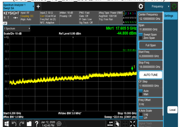
Plot 8-55. Conducted Spurious Emission Plot 6.2 GHz to 18 GHz
