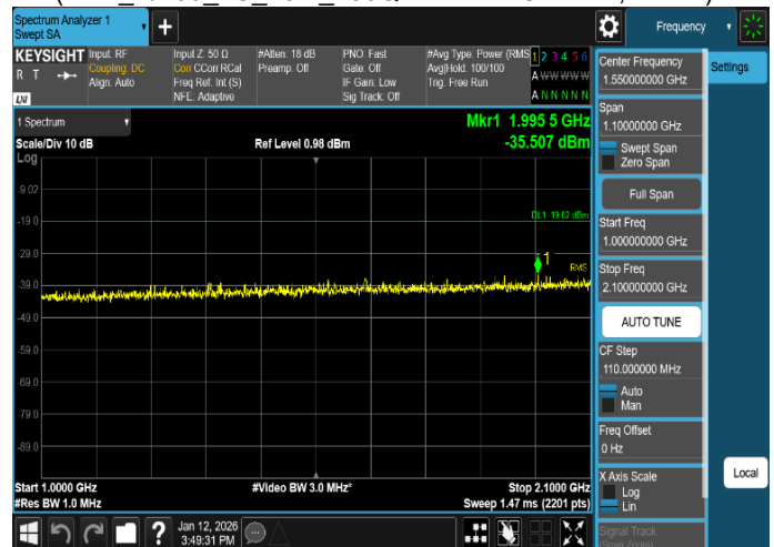
Plot 8-51. Conducted Spurious Emission Plot 1 GHz to 2.1 GHz
