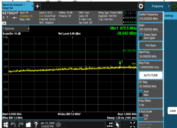
Plot 8-50. Conducted Spurious Emission Plot 30 MHz to 1 GHz
