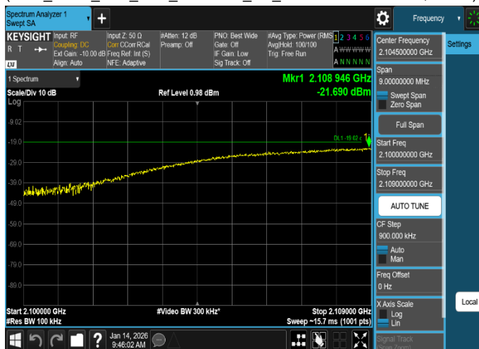
Plot 8-70. Conducted Spurious Emission Plot 2.1 GHz to 2.109 GHz
