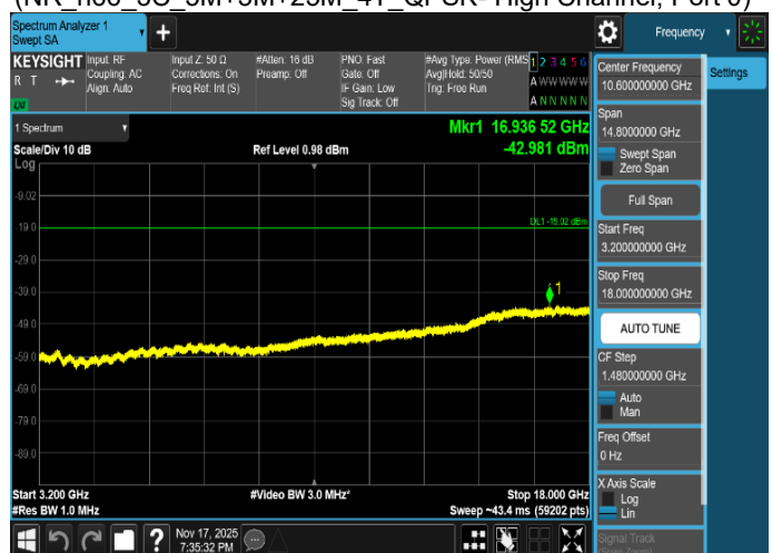
Plot 8-106. Conducted Spurious Emission Plot 3.2 GHz to 18 GHz
