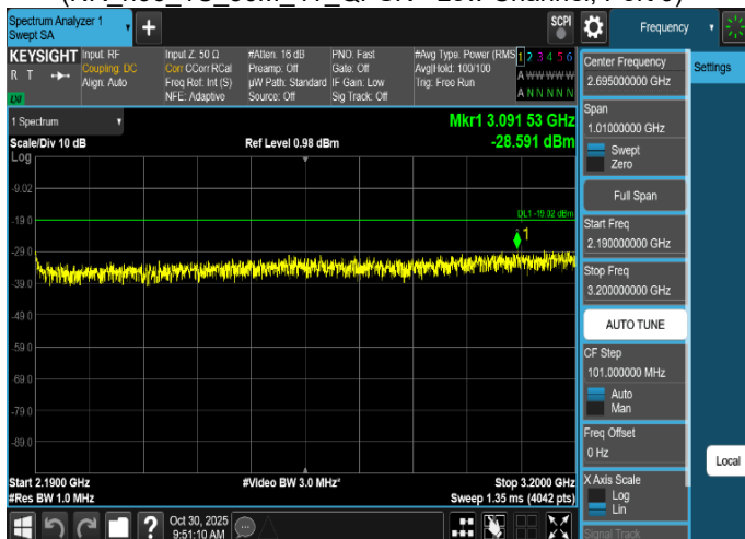
Plot 8-96. Conducted Spurious Emission Plot 2.190 GHz to 3.2 GHz
