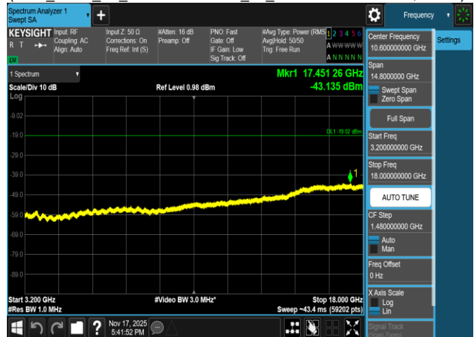
Plot 8-124. Conducted Spurious Emission Plot 3.2 GHz to 18 GHz
