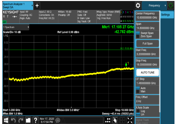
Plot 8-115. Conducted Spurious Emission Plot 3.2 GHz to 18 GHz
