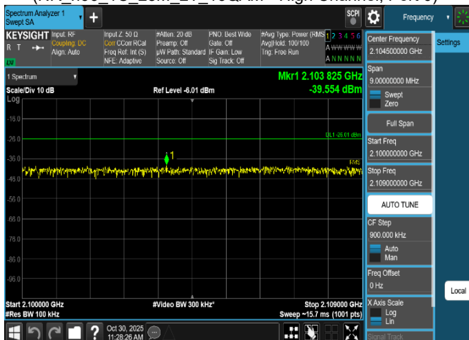
Plot 8-139. Conducted Spurious Emission Plot 2.1 GHz to 2.109 GHz
