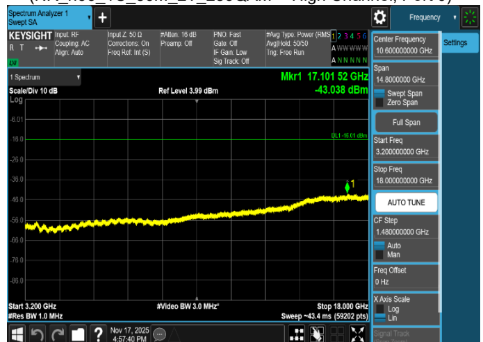
Plot 8-151. Conducted Spurious Emission Plot 3.2 GHz to 18 GHz
