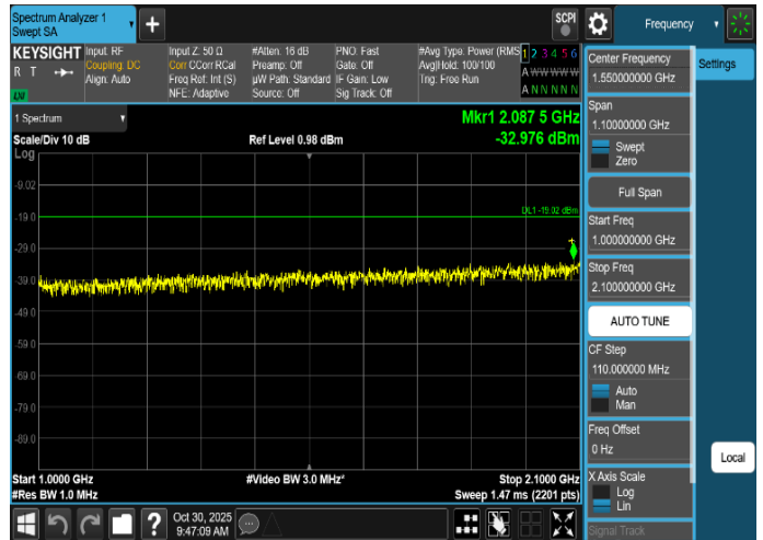
Plot 8-93. Conducted Spurious Emission Plot 1 GHz to 2.1 GHz
