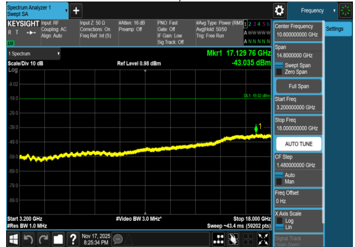
Plot 8-133. Conducted Spurious Emission Plot 3.2 GHz to 18 GHz
