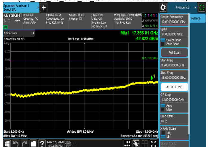
Plot 8-97. Conducted Spurious Emission Plot 3.2 GHz to 18 GHz
