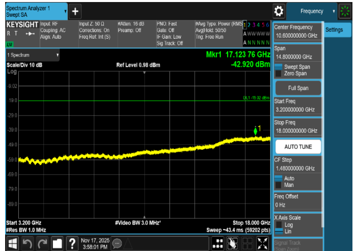
Plot 8-88. Conducted Spurious Emission Plot 3.2 GHz to 18 GHz (NR_n66_1C_25M_4T_QPSK - High Channel, Port 2)
