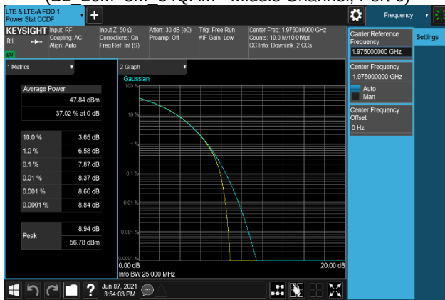
Plot 7-261. Peak To Average Power Ratio Plot (B2_20M+5M_QPSK - High Channel, Port 1)
