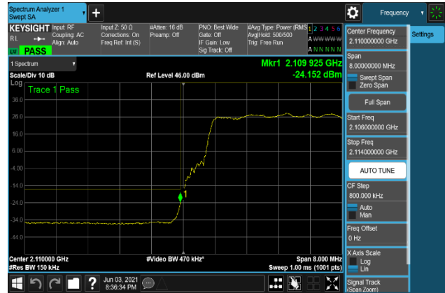
Plot 7-286. Band Edge Emission Plot 2109 MHz to 2110 MHz
