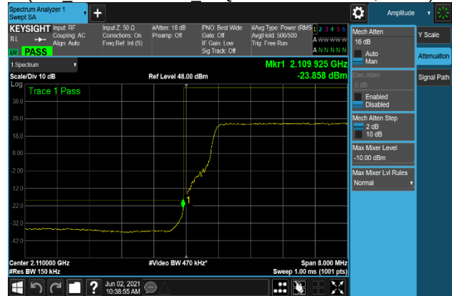
Plot 7-296. Band Edge Emission Plot 2109 MHz to 2110 MHz
