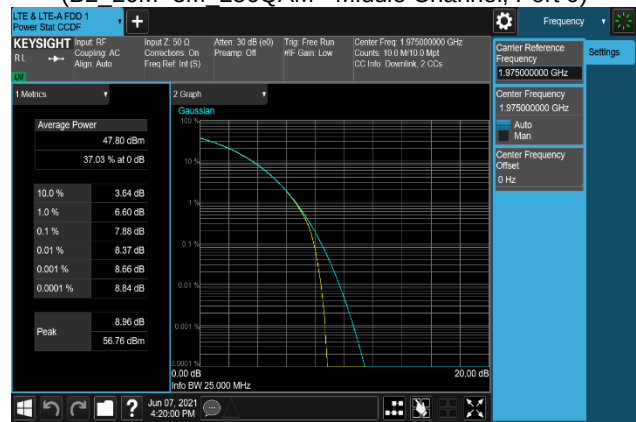
Plot 7-262. Peak To Average Power Ratio Plot (B2_20M+5M_16QAM - High Channel, Port 1)
