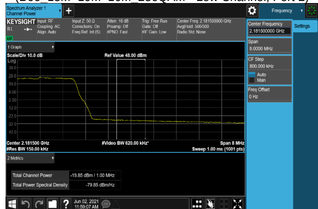
Plot 7-298. Band Edge Emission(Channel Power) Plot 2181 MHz to 2182 MHz
