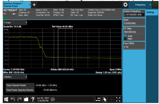
Plot 7-306. Band Edge Emission(Channel Power) Plot 2181 MHz to 2182 MHz (B66_15M+10M+10M_16QAM - High Channel, Port 1)
