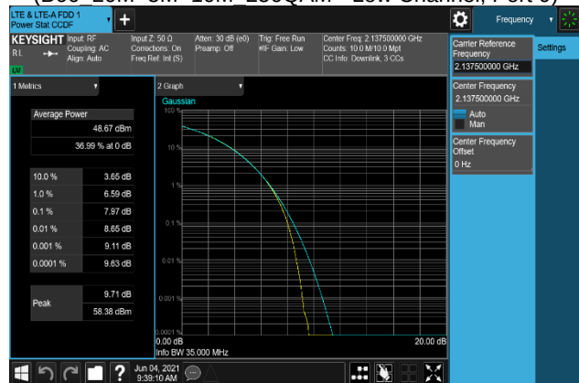
Plot 7-234. Peak To Average Power Ratio Plot (B66_20M+5M+10M_16QAM - Middle Channel, Port 0)
