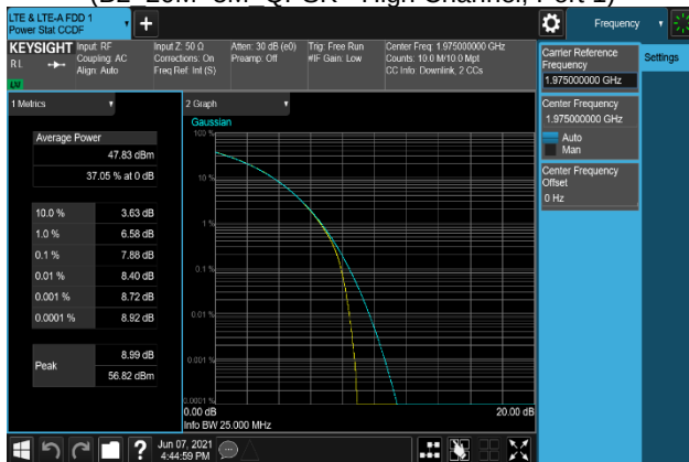
Plot 7-263. Peak To Average Power Ratio Plot (B2_20M+5M_64QAM - High Channel, Port 1)
