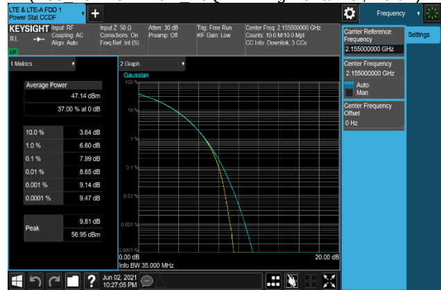
Plot 7-252. Peak To Average Power Ratio Plot (B66_20M+5M+10M_256QAM - High Channel, Port 0)
