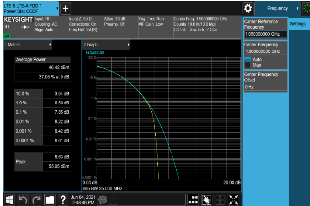
Plot 7-271. Peak To Average Power Ratio Plot (B2_20M+5M_64QAM - Middle Channel, Port 0)
