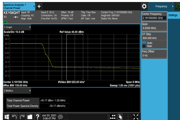
Plot 7-292. Band Edge Emission(Channel Power) Plot (2181 MHz to 2182 MHz (B66_15M+10M+10M_256QAM – High Channel, Port 0))
