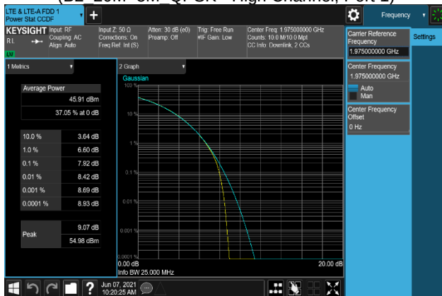
Plot 7-275. Peak To Average Power Ratio Plot (B2_20M+5M_64QAM - High Channel, Port 1)
