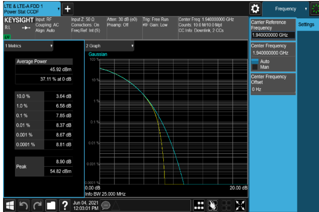
Plot 7-265. Peak To Average Power Ratio Plot (B2_20M+5M_QPSK - Low Channel, Port 3)
