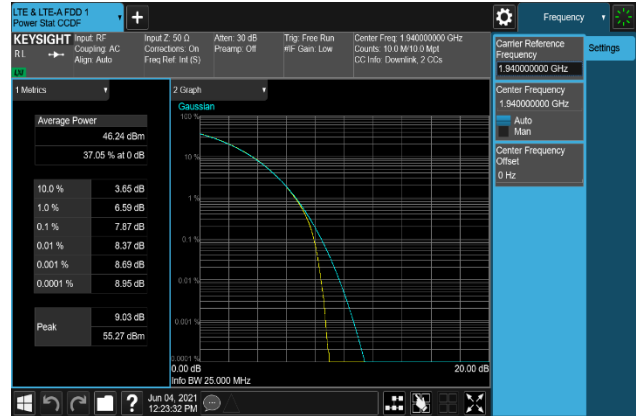
Plot 7-266. Peak To Average Power Ratio Plot (B2_20M+5M_16QAM - Low Channel, Port 1)
