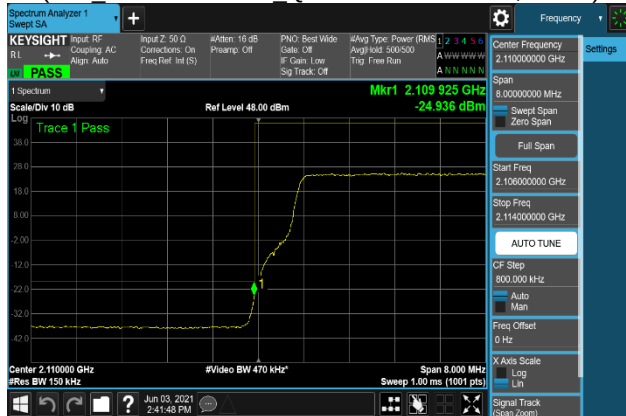
Plot 7-295. Band Edge Emission Plot 2109 MHz to 2110 MHz
