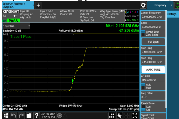
Plot 7-279. Band Edge Emission Plot 2109 MHz to 2110 MHz
