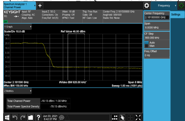
Plot 7-290. Band Edge Emission(Channel Power) Plot 2181 MHz to 2182 MHz
