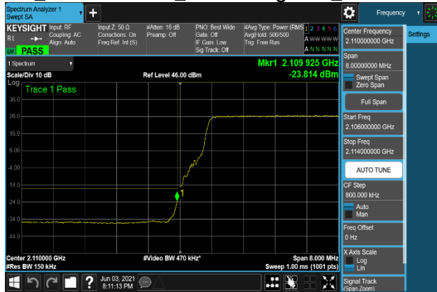
Plot 7-285. Band Edge Emission Plot 2109 MHz to 2110 MHz
