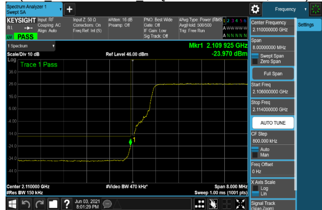
Plot 7-280. Band Edge Emission Plot 2109 MHz to 2110 MHz
