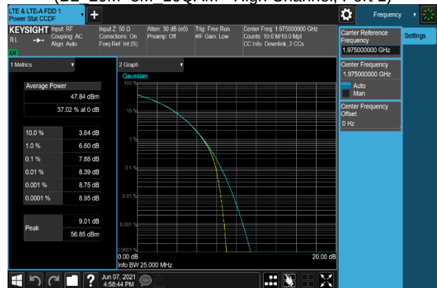
Plot 7-264. Peak To Average Power Ratio Plot (B2_20M+5M_256QAM - High Channel, Port 1)
