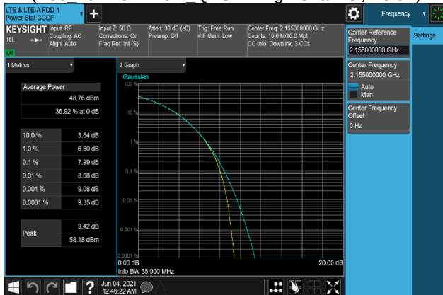
Plot 7-239. Peak To Average Power Ratio Plot (B66_20M+5M+10M_64QAM - High Channel, Port 1)
