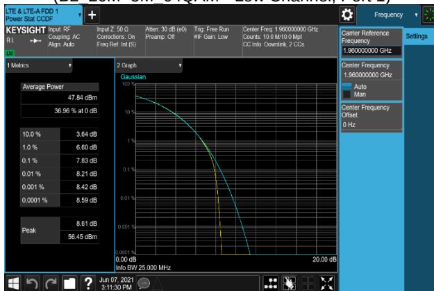
Plot 7-257. Peak To Average Power Ratio Plot (B2_20M+5M_QPSK - Middle Channel, Port 0)
