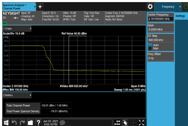
Plot 7-291. Band Edge Emission(Channel Power) Plot (2181 MHz to 2182 MHz (B66_15M+10M+10M_64QAM – High Channel, Port 0))
