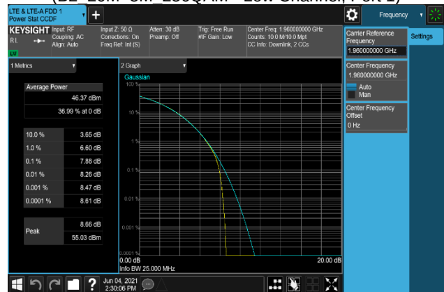
Plot 7-270. Peak To Average Power Ratio Plot (B2_20M+5M_16QAM - Middle Channel, Port 0)
