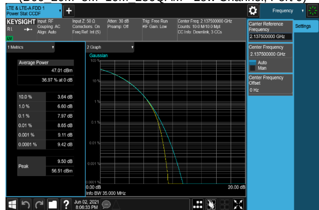
Plot 7-246. Peak To Average Power Ratio Plot (B66_20M+5M+10M_16QAM - Middle Channel, Port 1)
