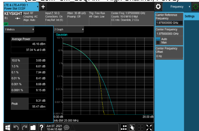
Plot 7-276. Peak To Average Power Ratio Plot (B2_20M+5M_256QAM - High Channel, Port 1)
