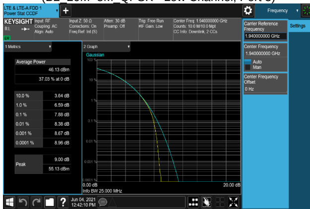
Plot 7-267. Peak To Average Power Ratio Plot (B2_20M+5M_64QAM - Low Channel, Port 1)
