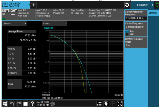
Plot 7-251. Peak To Average Power Ratio Plot (B66_20M+5M+10M_64QAM - High Channel, Port 1)
