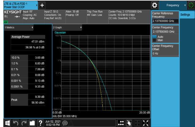
Plot 7-248. Peak To Average Power Ratio Plot (B66_20M+5M+10M_256QAM - Middle Channel, Port 3)
