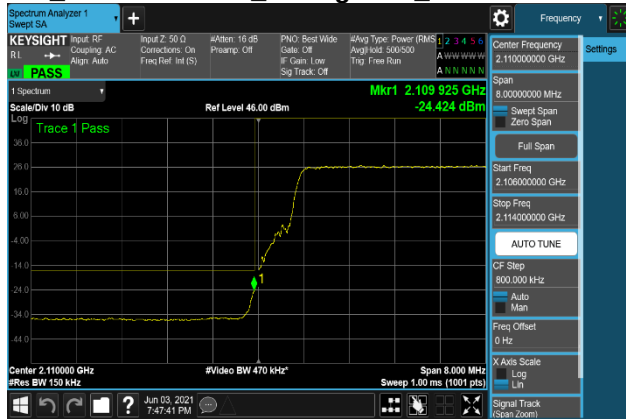
Plot 7-277. Band Edge Emission Plot 2109 MHz to 2110 MHz
