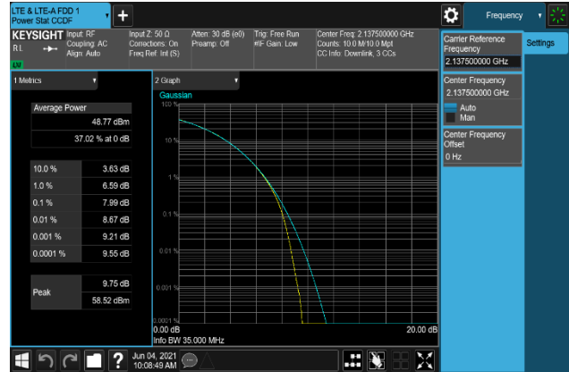
Plot 7-236. Peak To Average Power Ratio Plot (B66_20M+5M+10M_256QAM - Middle Channel, Port 1)
