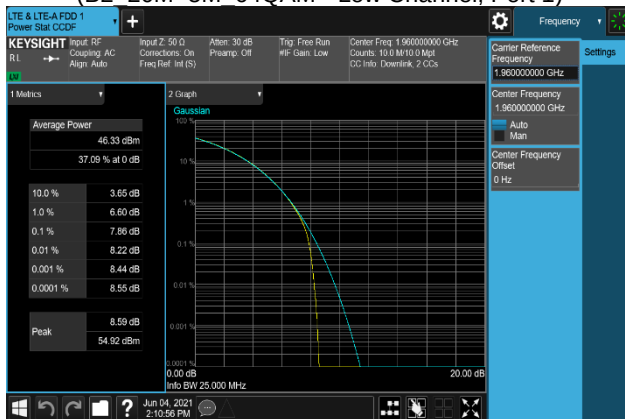
Plot 7-269. Peak To Average Power Ratio Plot (B2_20M+5M_QPSK - Middle Channel, Port 0)
