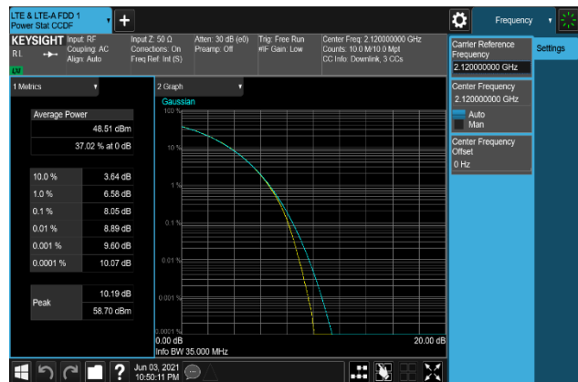
Plot 7-230. Peak To Average Power Ratio Plot (B66_20M+5M+10M_16QAM - Low Channel, Port 0)
