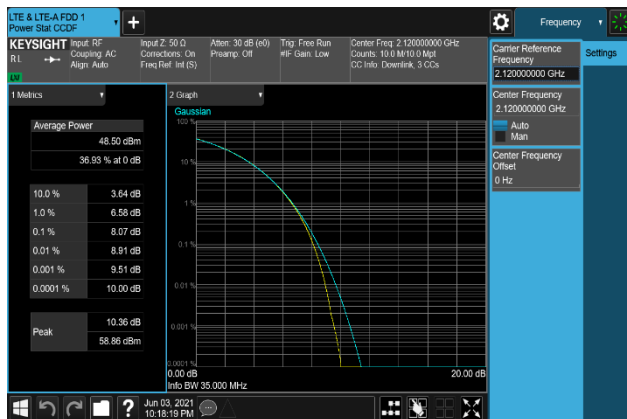
Plot 7-229. Peak To Average Power Ratio Plot (B66_20M+5M+10M_QPSK - Low Channel, Port 0)
