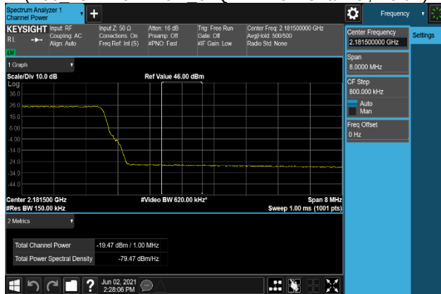
Plot 7-305. Band Edge Emission(Channel Power) Plot 2181 MHz to 2182 MHz (B66_15M+10M+10M_QPSK - High Channel, Port 1)
