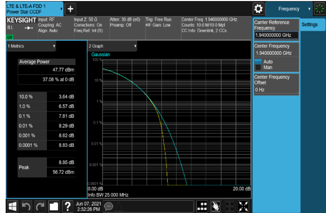
Plot 7-254. Peak To Average Power Ratio Plot (B2_20M+5M_16QAM - Low Channel, Port 1)
