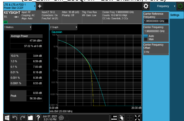
Plot 7-258. Peak To Average Power Ratio Plot (B2_20M+5M_16QAM - Middle Channel, Port 0)
