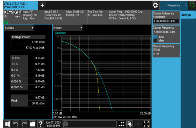
Plot 7-260. Peak To Average Power Ratio Plot (B2_20M+5M_256QAM - Middle Channel, Port 0)
