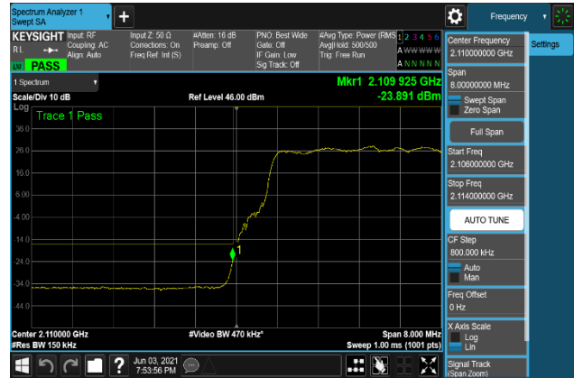
Plot 7-278. Band Edge Emission Plot 2109 MHz to 2110 MHz
