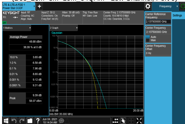
Plot 7-233. Peak To Average Power Ratio Plot (B66_20M+5M+10M_QPSK - Middle Channel, Port 0)
