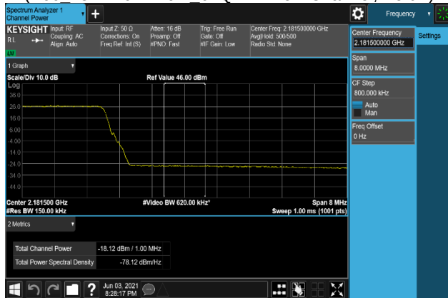
Plot 7-289. Band Edge Emission(Channel Power) Plot 2181 MHz to 2182 MHz
