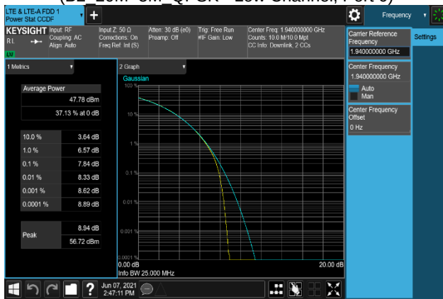
Plot 7-255. Peak To Average Power Ratio Plot (B2_20M+5M_64QAM - Low Channel, Port 1)
