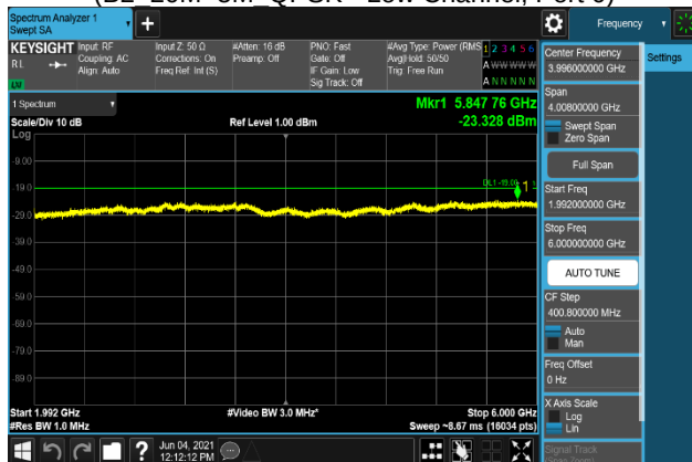
Plot 7-517. Conducted Spurious Emission Plot 1.992 GHz to 6 GHz (B2_20M+5M_QPSK - Low Channel, Port 0)
