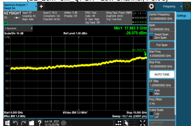
Plot 7-518. Conducted Spurious Emission Plot 6 GHz to 18 GHz (B2_20M+5M_QPSK - Low Channel, Port 0)
