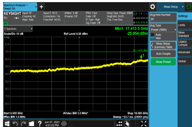
Plot 7-504. Conducted Spurious Emission Plot 6 GHz to 18 GHz (B2_20M+5M_QPSK - High Channel, Port 0)
