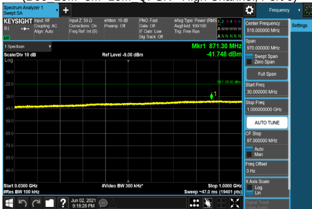
Plot 7-473. Conducted Spurious Emission Plot 30 MHz to 1 GHz
