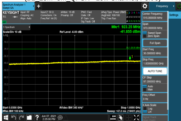
Plot 7-487. Conducted Spurious Emission Plot 30 MHz to 1 GHz (B2_20M+5M_QPSK - Low Channel, Port 0)
