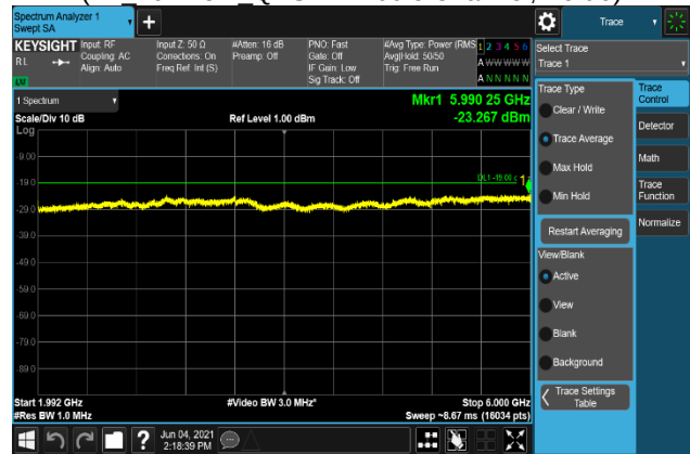
Plot 7-524. Conducted Spurious Emission Plot 1.992 GHz to 6 GHz (B2_20M+5M_QPSK - Middle Channel, Port 0)
