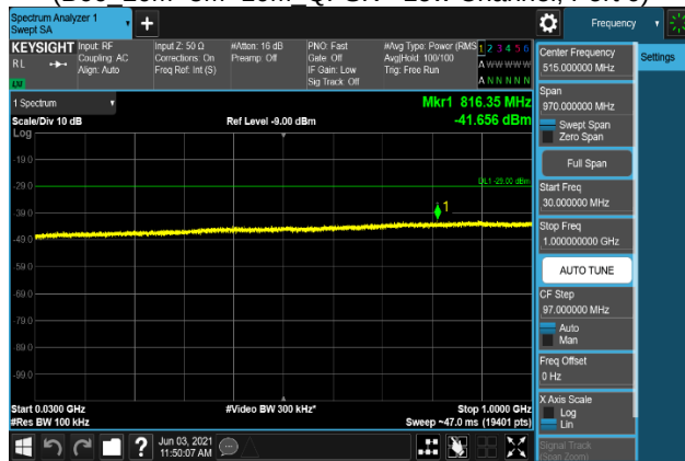
Plot 7-480. Conducted Spurious Emission Plot 30 MHz to 1 GHz (B66_20M+5M+10M_QPSK - Low Channel, Port 0)
