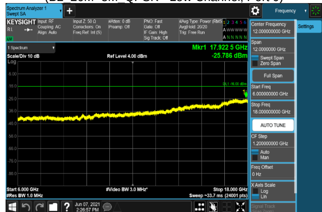
Plot 7-490. Conducted Spurious Emission Plot 6 GHz to 18 GHz (B2_20M+5M_QPSK - Low Channel, Port 0)
