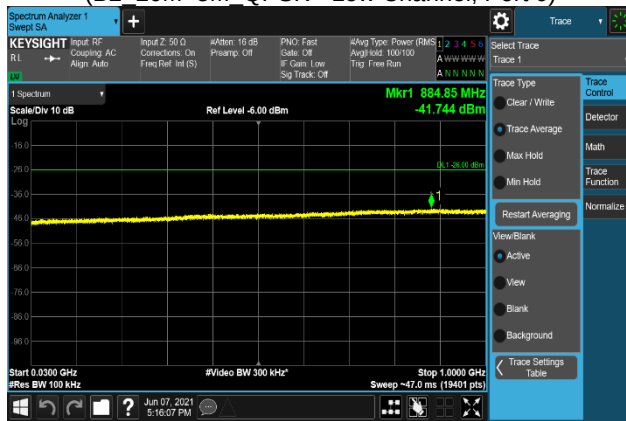
Plot 7-508. Conducted Spurious Emission Plot 30 MHz to 1 GHz (B2_20M+5M_QPSK - Low Channel, Port 0)
