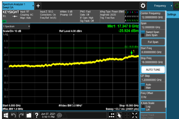
Plot 7-497. Conducted Spurious Emission Plot 6 GHz to 18 GHz (B2 20M+5M_QPSK - Middle Channel, Port 0)
