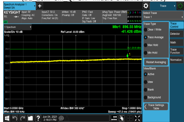
Plot 7-522. Conducted Spurious Emission Plot 30 MHz to 1 GHz (B2 20M+5M_QPSK - Middle Channel, Port 0)
