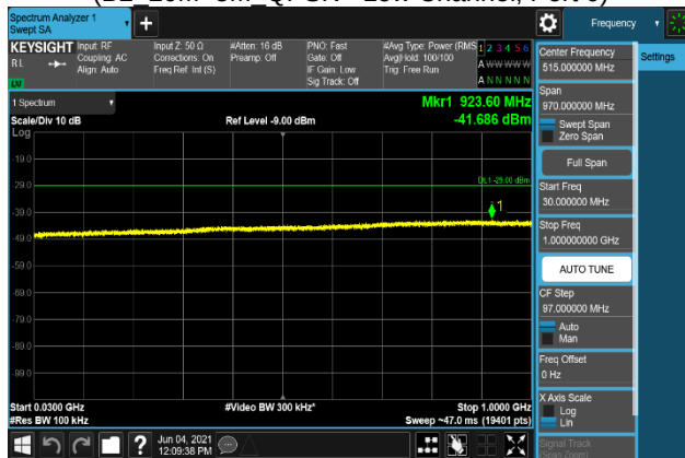
Plot 7-515. Conducted Spurious Emission Plot 30 MHz to 1 GHz (B2_20M+5M_QPSK - Low Channel, Port 0)
