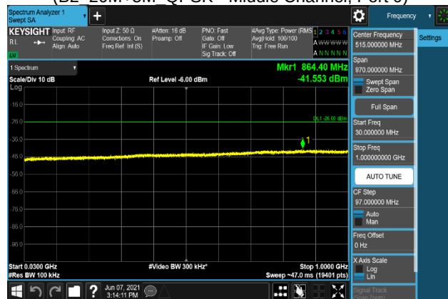
Plot 7-494. Conducted Spurious Emission Plot 30 MHz to 1 GHz (B2_20M+5M_QPSK - Middle Channel, Port 0)
