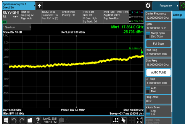
Plot 7-469. Conducted Spurious Emission Plot 6 GHz to 18 GHz
