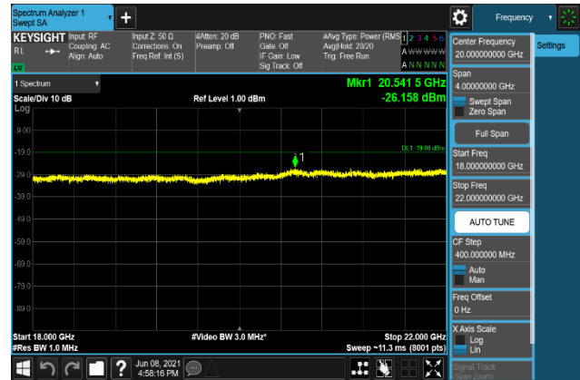
Plot 7-470. Conducted Spurious Emission Plot 18 GHz to 22 GHz
