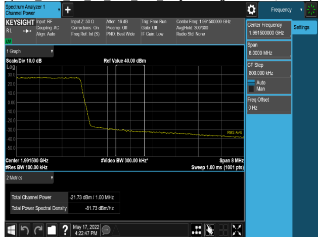
Plot 8-330. Band Edge Emission Plot (PCS_NR_1C_5M+LTE_1C_5M_4TX_QPSK - High Channel, Port 0)
