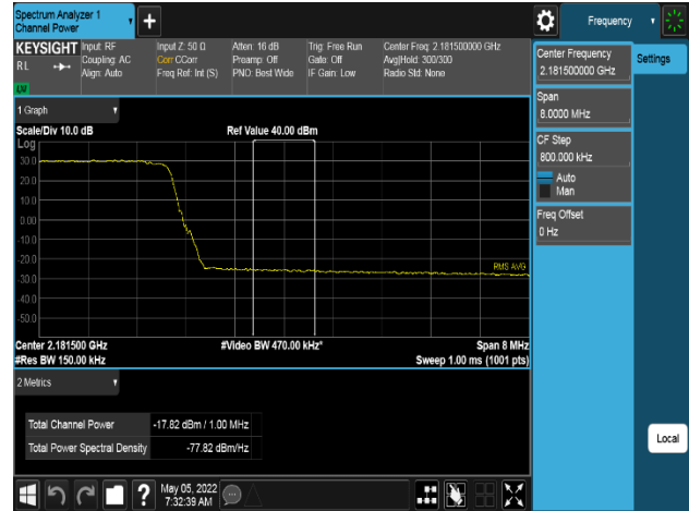
Plot 8-310. Band Edge Emission Plot (AWS DSS 2:8 1C 15M 2TX 64QAM - High Channel, Port 0)
