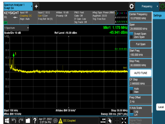
Plot 8-378. Conducted Spurious Emission Plot 150 kHz to 30 MHz (AWS_NR_1C_5M_2TX_256QAM - High Channel, Port 0)
