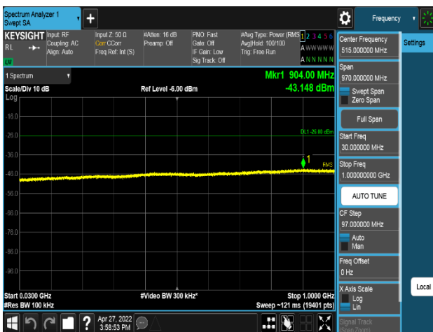
Plot 8-379. Conducted Spurious Emission Plot 30 MHz to 1 GHz (AWS_NR_1C_5M_2TX_256QAM - High Channel, Port 0)
