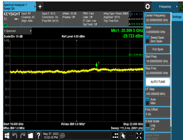
Plot 8-362. Conducted Spurious Emission Plot 18 GHz to 22 GHz (PCS_DSS_2:8_1C_20M_2TX_16QAM - High Channel, Port 0)
