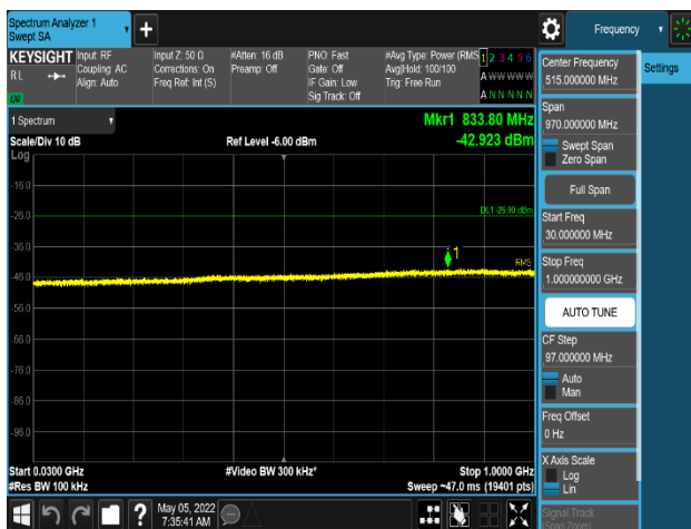
Plot 8-358. Conducted Spurious Emission Plot 30 MHz to 1 GHz (PCS_DSS_2:8_1C_20M_2TX_16QAM - High Channel, Port 0)
