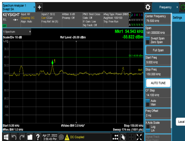
Plot 8-377. Conducted Spurious Emission Plot 9 kHz to 150 kHz (AWS_NR_1C_5M_2TX_256QAM - High Channel, Port 0)
