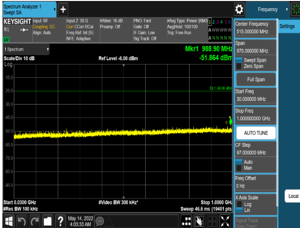
Plot 8-386. Peak To Average Power Ratio Plot 30 MHz to 1 GHz (AWS_DSS_9:1_1C_20M_2TX_QPSK - High Channel, Port 1)
