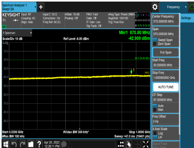
Plot 8-351. Conducted Spurious Emission Plot 30 MHz to 1 GHz (PCS_NR_1C_5M_2TX_64QAM - Low Channel, Port 0)
