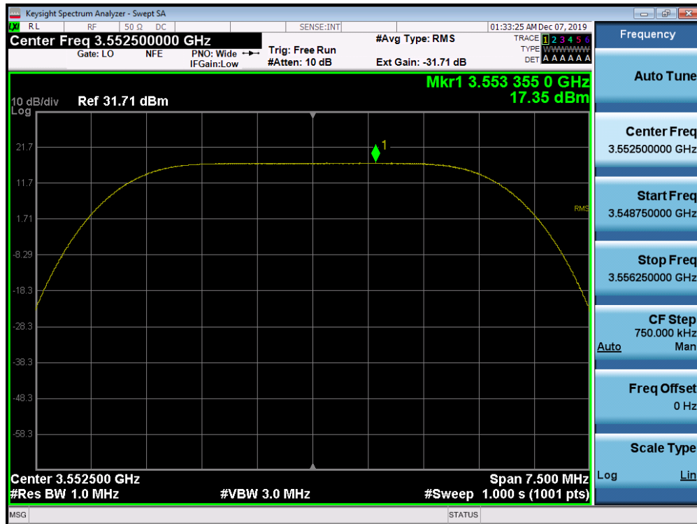
Plot 7-69. Peak Power Spectral Density Plot (1CC Configuration 5MHz 64QAM - Low Channel) Port 00
