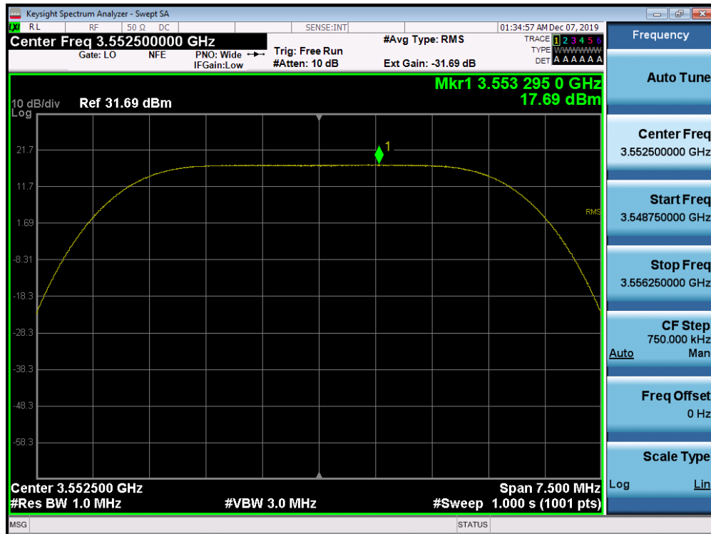
Plot 7-71. Peak Power Spectral Density Plot (1CC Configuration 5MHz 64QAM - Low Channel) Port 02
