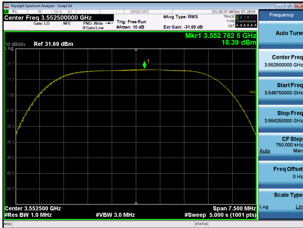
Plot 7-67. Peak Power Spectral Density Plot (1CC Configuration 5MHz 16QAM - Low Channel) Port 02
