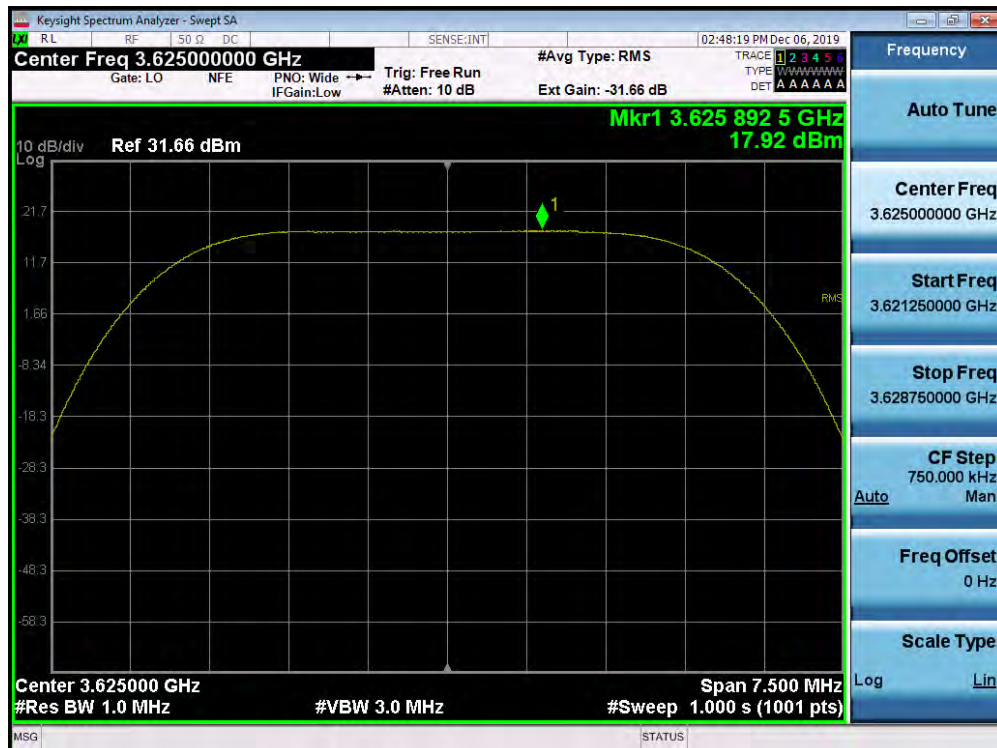
Plot 7-80. Peak Power Spectral Density Plot (1CC Configuration 5MHz QPSK - Mid Channel) Port 03
