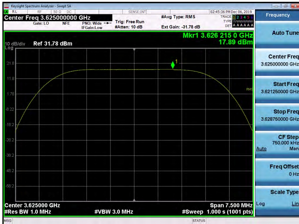
Plot 7-78. Peak Power Spectral Density Plot (1CC Configuration 5MHz QPSK - Mid Channel) Port 01
