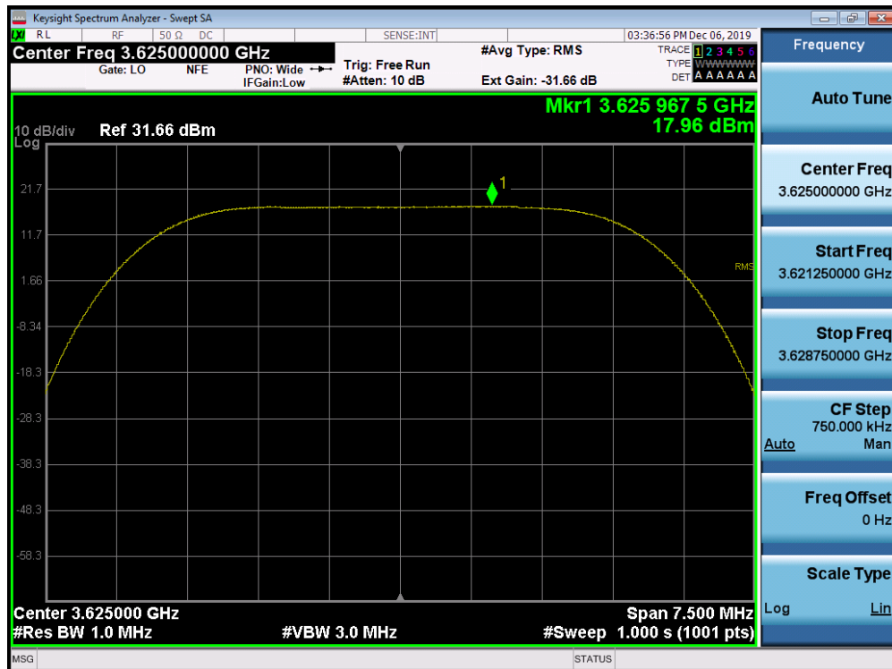
Plot 7-88. Peak Power Spectral Density Plot (1CC Configuration 5MHz 64QAM - Mid Channel) Port 03
