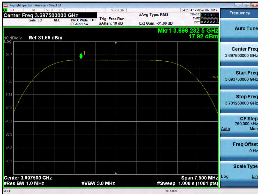
Plot 7-96. Peak Power Spectral Density Plot (1CC Configuration 5MHz QPSK - High Channel) Port 03
