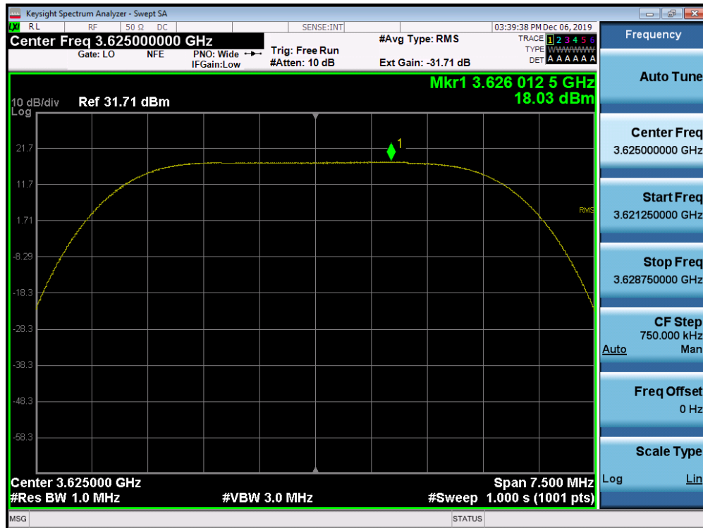
Plot 7-89. Peak Power Spectral Density Plot (1CC Configuration 5MHz 256QAM - Mid Channel) Port 00
