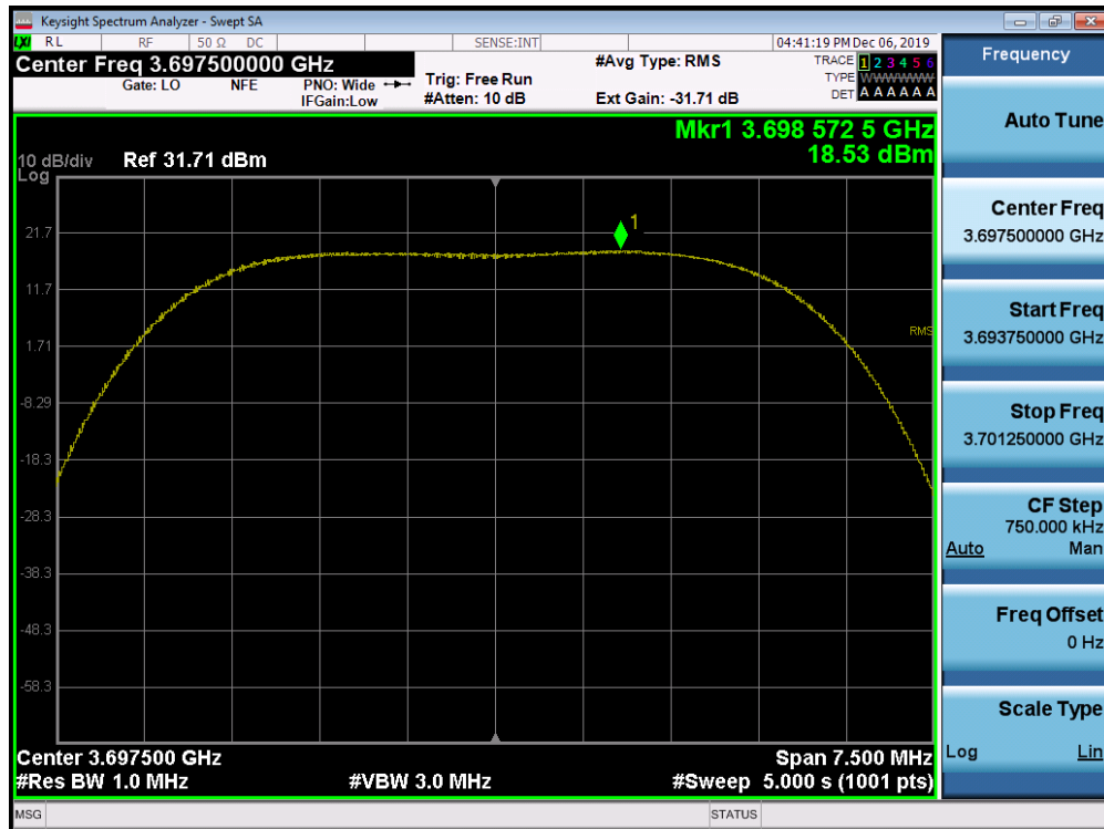
Plot 7-97. Peak Power Spectral Density Plot (1CC Configuration 5MHz 16QAM - High Channel) Port 00
