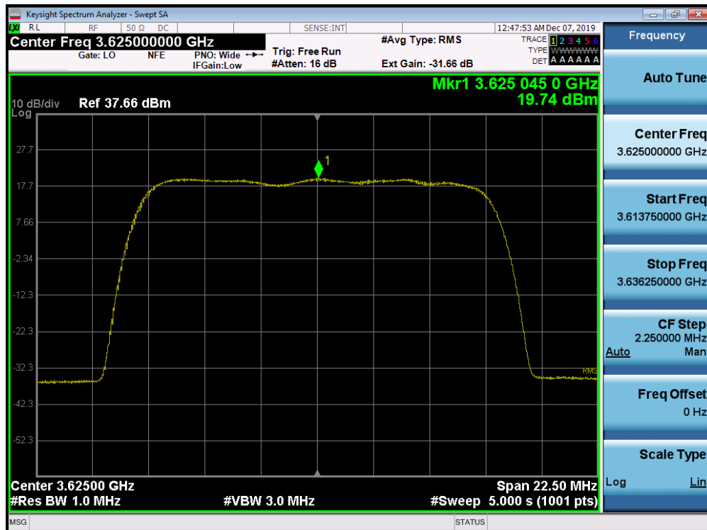
Plot 7-132. Peak Power Spectral Density Plot (1CC Configuration 15MHz 16QAM - Mid Channel) Port 03
