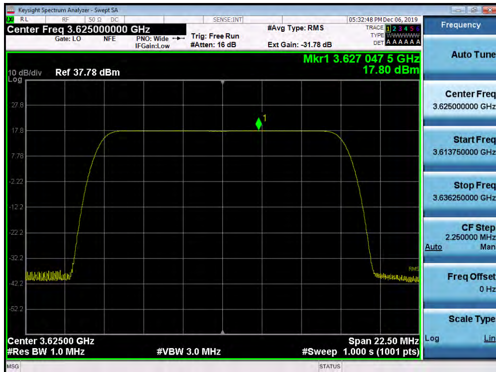
Plot 7-126. Peak Power Spectral Density Plot (1CC Configuration 15MHz QPSK - Mid Channel) Port 01
