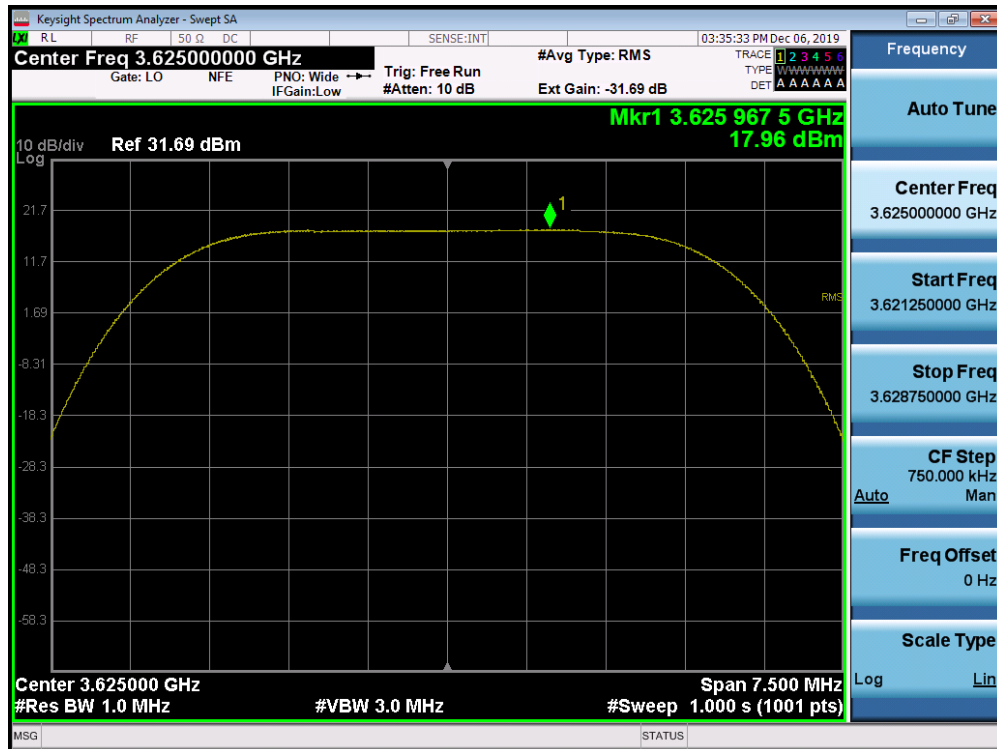
Plot 7-87. Peak Power Spectral Density Plot (1CC Configuration 5MHz 64QAM - Mid Channel) Port 02
