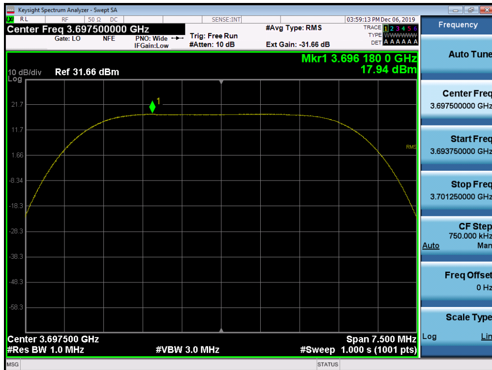
Plot 7-108. Peak Power Spectral Density Plot (1CC Configuration 5MHz 256QAM - High Channel) Port 03
