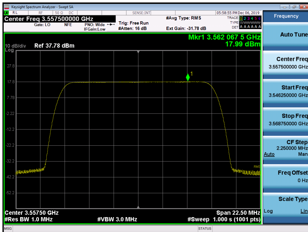
Plot 7-118. Peak Power Spectral Density Plot (1CC Configuration 15MHz 64QAM - Low Channel) Port 01
