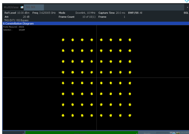
Plot 8-45. Modulation Characteristics Plot (NR_n48_1C_10M_64QAM Modulation)
