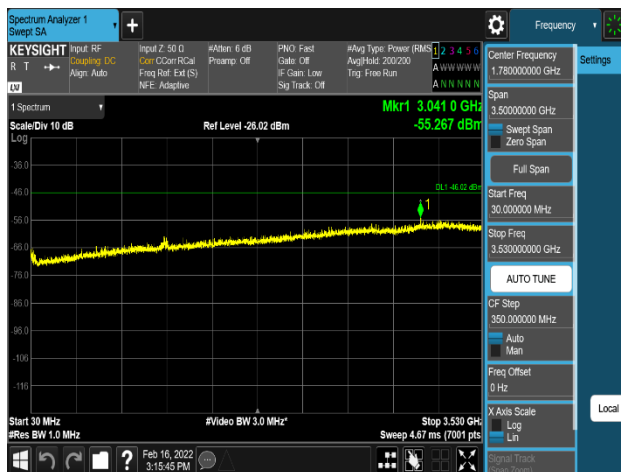
Plot 8-284. Conducted Spurious Emission Plot 30 MHz to 3530 MHz (LTE_2C+NR_1C_20M+40M+40M_64QAM- Mid Channel, Port 3)
