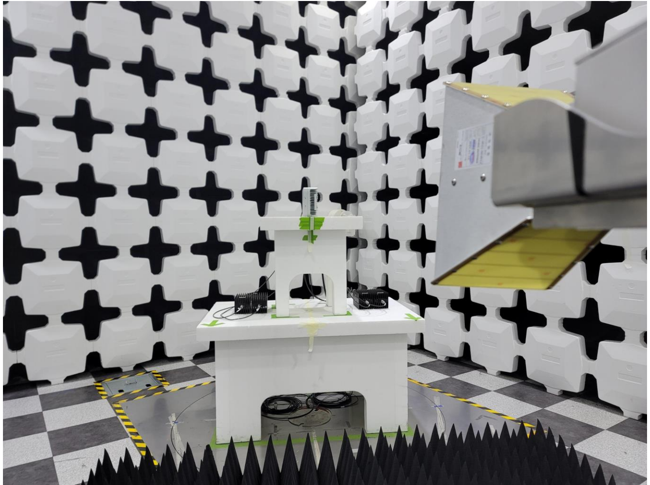
Above 1GHz Test Instrument & Measurement Setup > 1GHz
