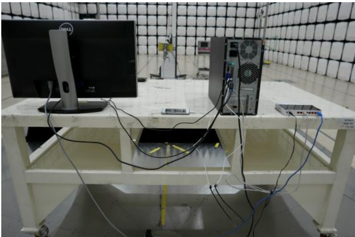
[ Radiated Disturbance for Above 1 GHz – Rear ]
