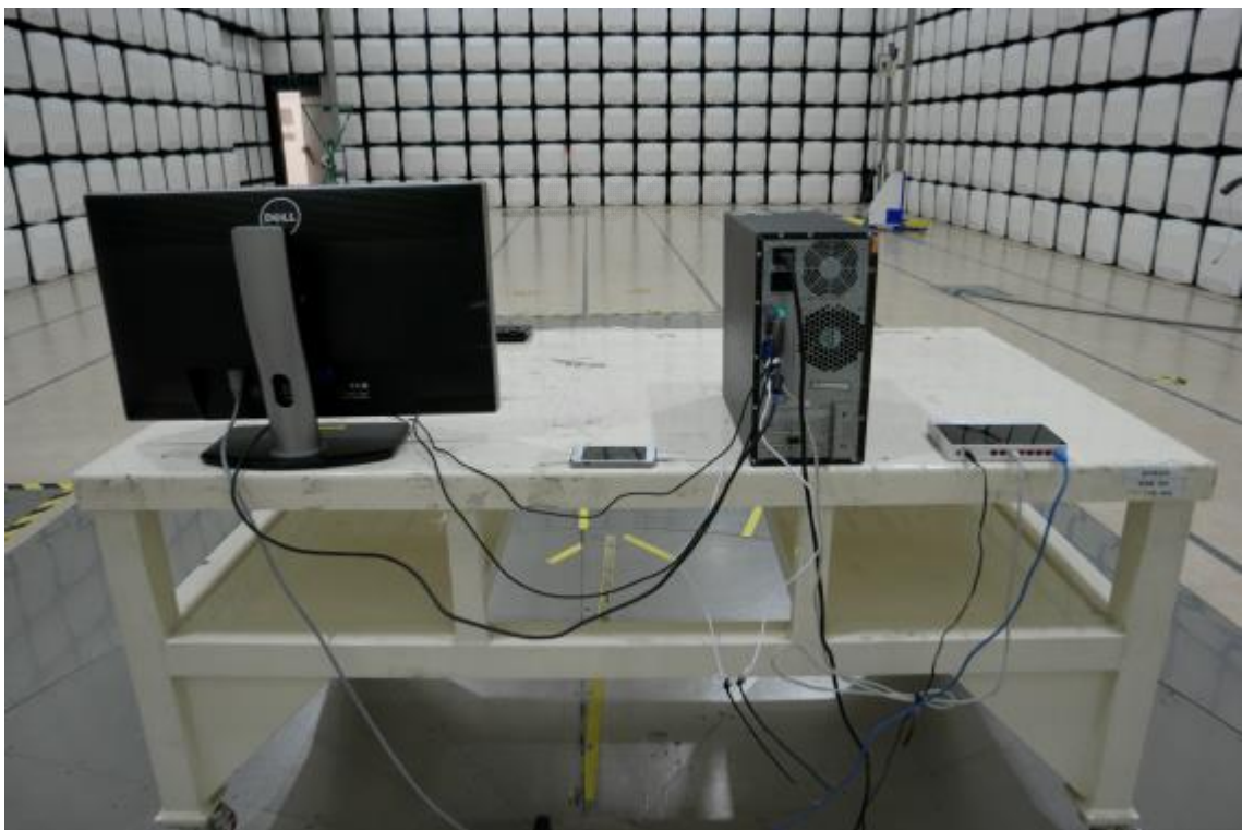
[ Radiated Disturbance for Below 1 GHz – Rear ]
