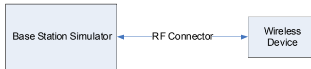
Figure 9-1 Power Measurement Setup
