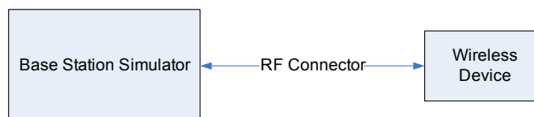
Figure 9-2 Power Measurement Setup
