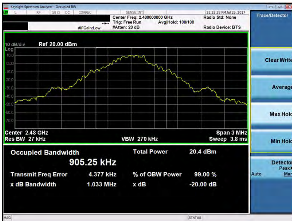
Plot 7-3. 20dB Bandwidth Plot (Bluetooth, 1Mbps – Ch. 78)
