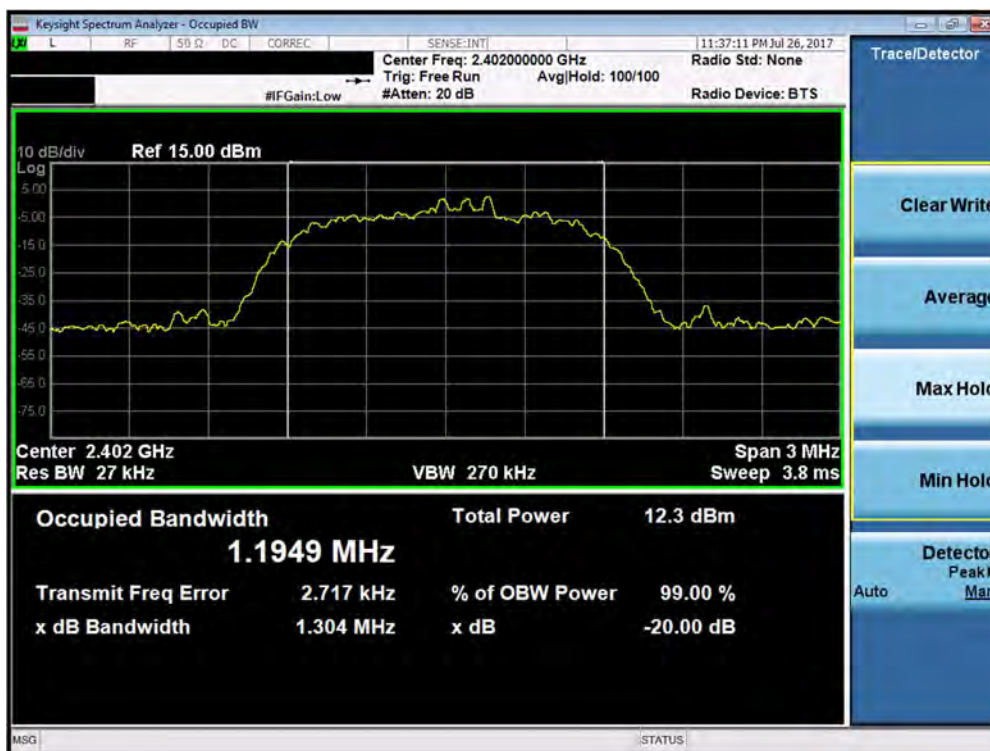
Plot 7-7. 20dB Bandwidth Plot (Bluetooth, 3Mbps – Ch. 0)
