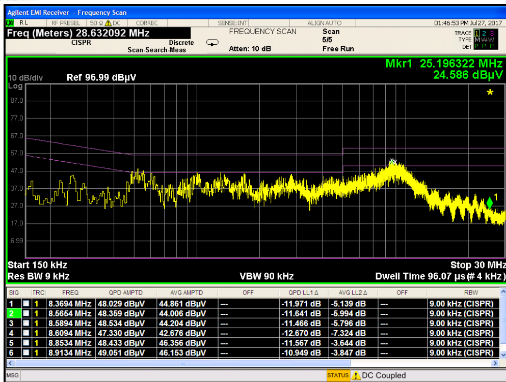
Plot 7-286. Line Conducted Plot with 802.11a UNII Band 2A (L1)
