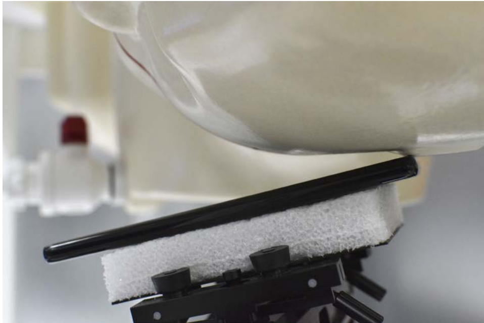
SAR Test Setup Photo 4 – Left Tilt
