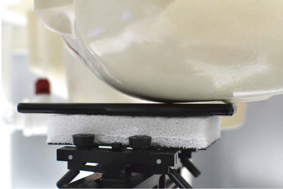
SAR Test Setup Photo 3 – Left Cheek
