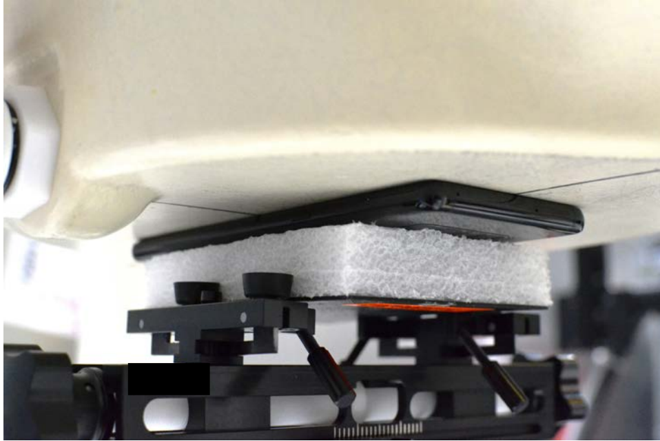
SAR Test Setup Photo 9 – Front Side at 0 mm
