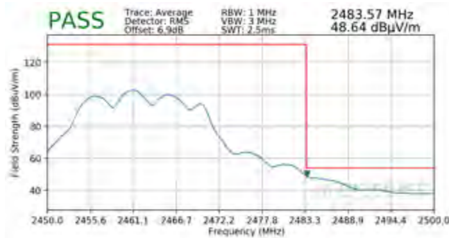
Plot 7-121. Radiated Restricted Band Edge Measurement CDD with WCP (Average)
