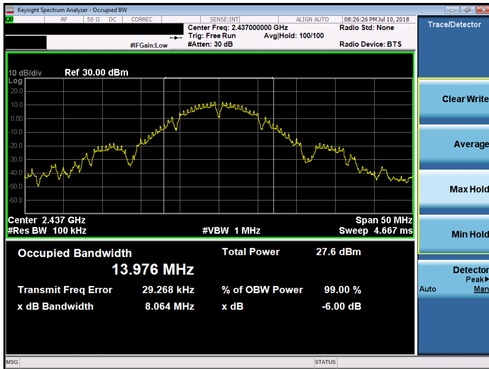
Plot 7-11. 6dB Bandwidth Plot SISO ANT1 (802.11b – Ch. 6)
