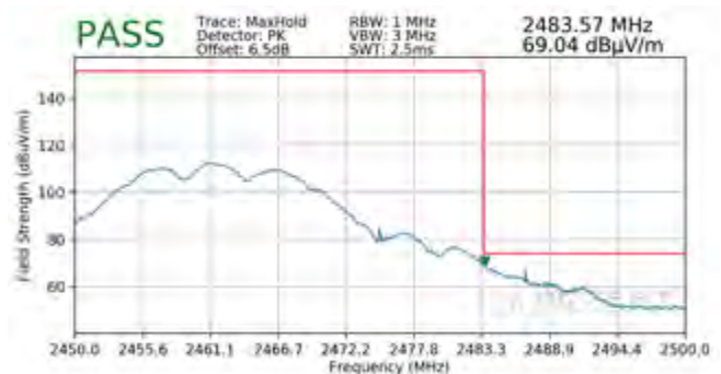
Plot 7-120. Radiated Restricted Upper Band Edge Measurement CDD (Peak)
