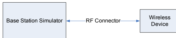
Figure 9-2 Power Measurement Setup
