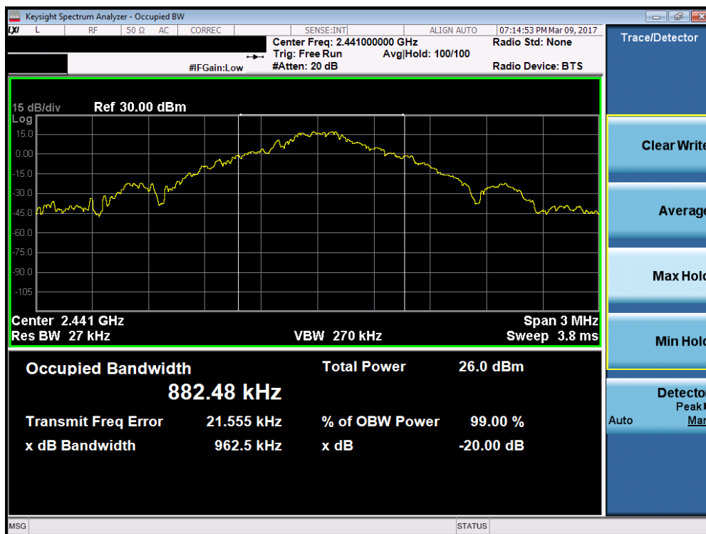
Plot 7-2. 20dB Bandwidth Plot (Bluetooth, 1Mbps – Ch. 39)
