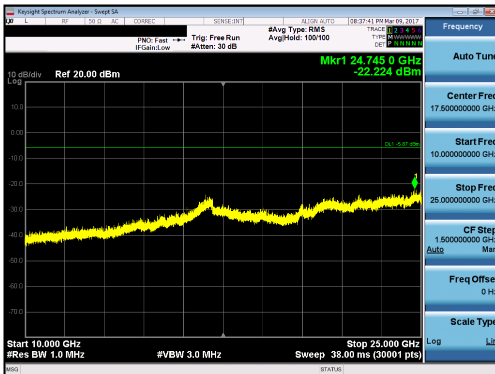
Plot 7-39. Conducted Spurious Plot (Bluetooth, 1Mbps – Ch. 39)
