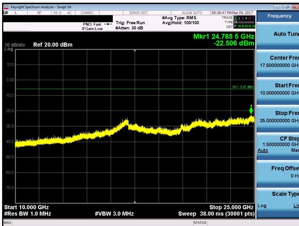
Plot 7-41. Conducted Spurious Plot (Bluetooth, 1Mbps – Ch. 78)
