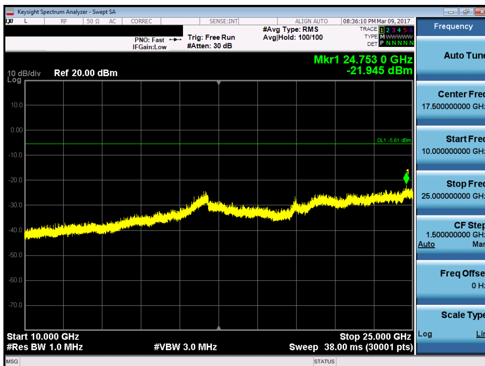
Plot 7-37. Conducted Spurious Plot (Bluetooth, 1Mbps – Ch. 0)
