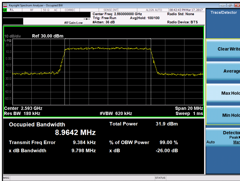
Plot 7-35. Occupied Bandwidth Plot (Band 41 – 10.0MHz QPSK – RB Size 50)
