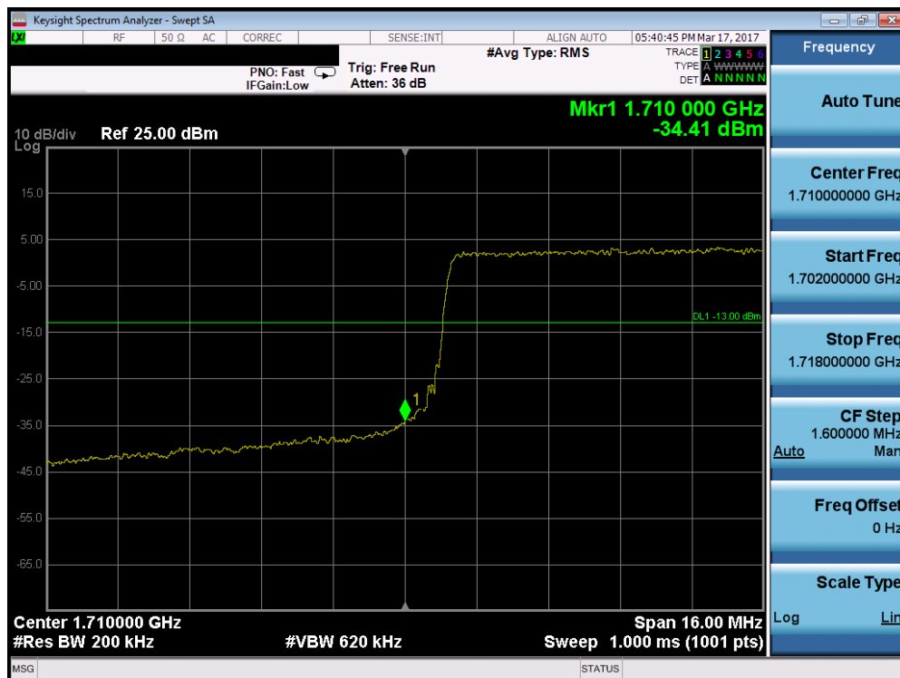
Plot 7-124. Lower Band Edge Plot (Band 4 – 20.0MHz QPSK – RB Size 100)
