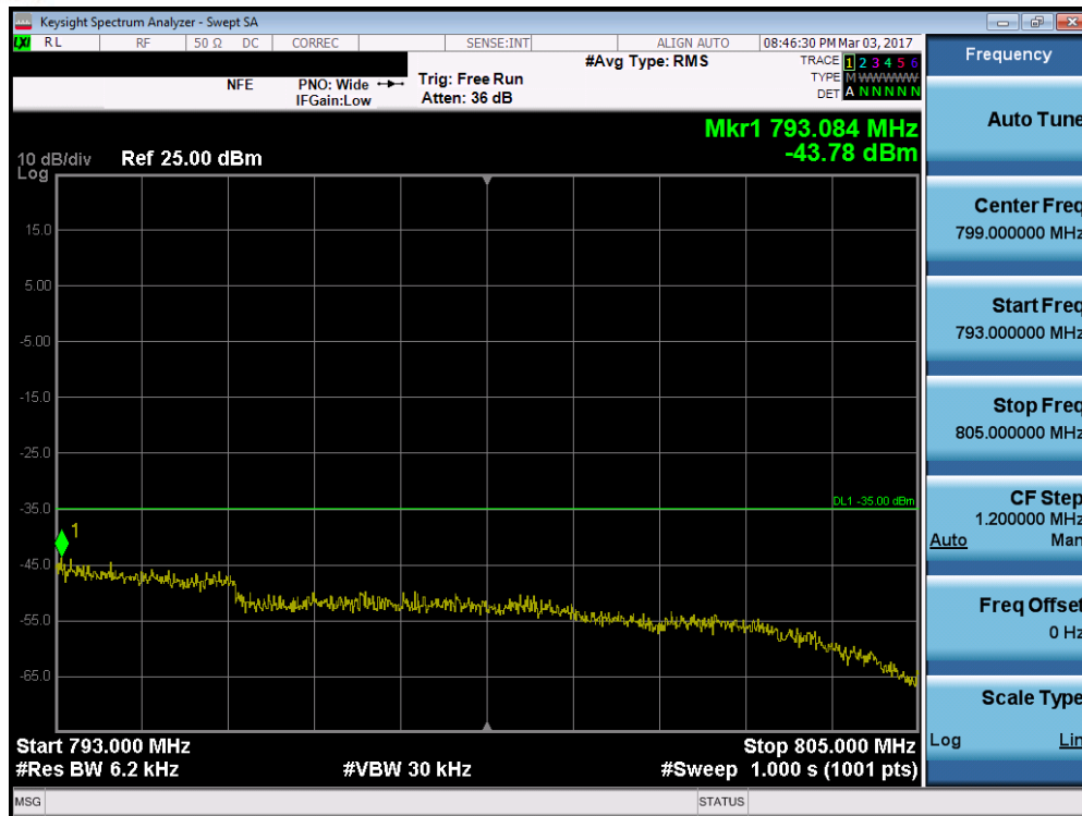
Plot 7-95. Upper Emission Mask Edge Plot (Band 13 – 10.0MHz QPSK – RB Size 50)
