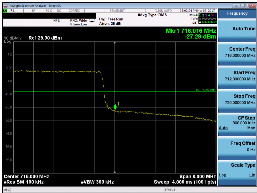
Plot 7-87. Upper Band Edge Plot (Band 12/17 – 10.0MHz QPSK – RB Size 50)
