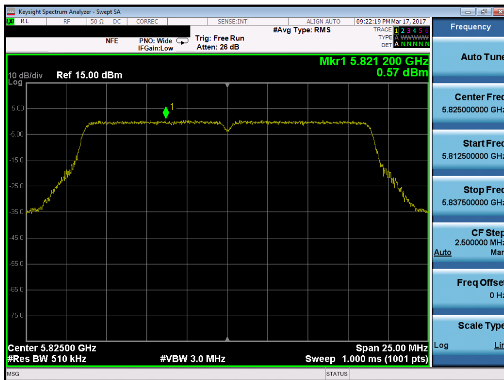
Plot 7-153. Power Spectral Density Plot (20MHz BW 802.11n (UNII Band 3) – Ch. 165)
