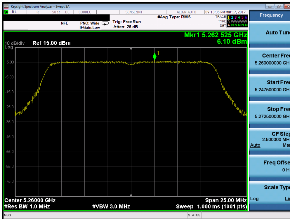
Plot 7-130. Power Spectral Density Plot (20MHz BW 802.11n (UNII Band 2A) – Ch. 52)
