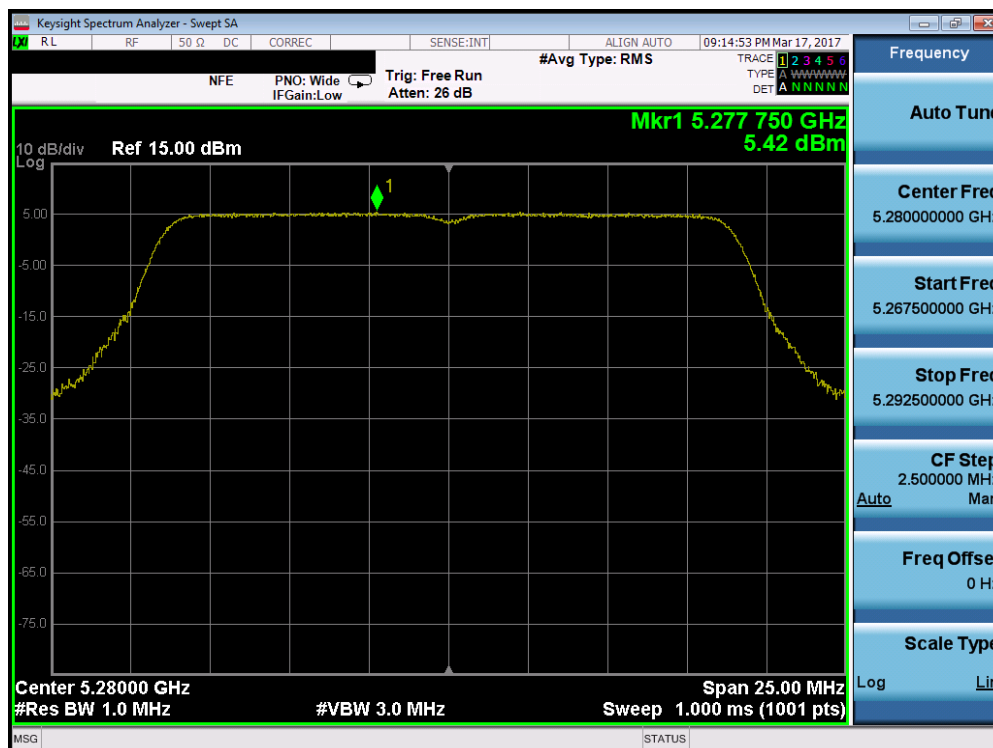
Plot 7-131. Power Spectral Density Plot (20MHz BW 802.11n (UNII Band 2A) – Ch. 56)
