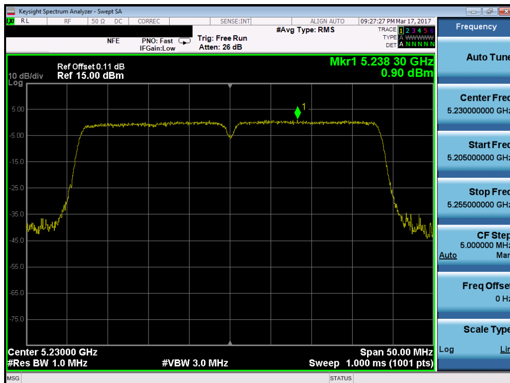
Plot 7-125. Power Spectral Density Plot (40MHz BW 802.11n (UNII Band 1) – Ch. 46)
