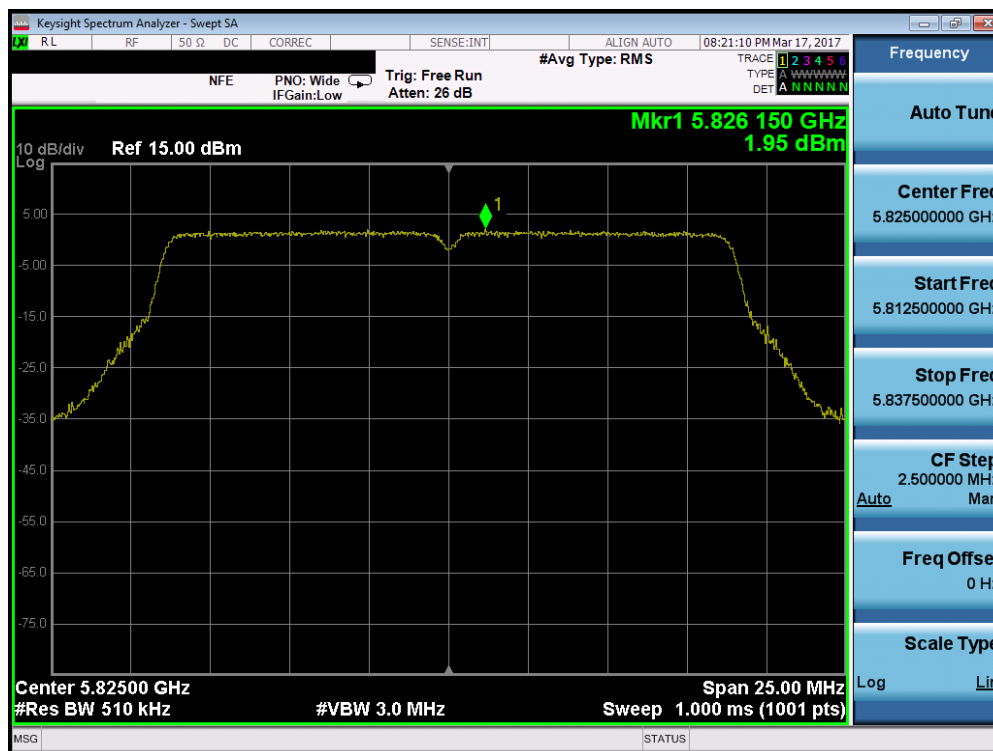
Plot 7-114. Power Spectral Density Plot (20MHz BW 802.11n (UNII Band 3) – Ch. 165)
