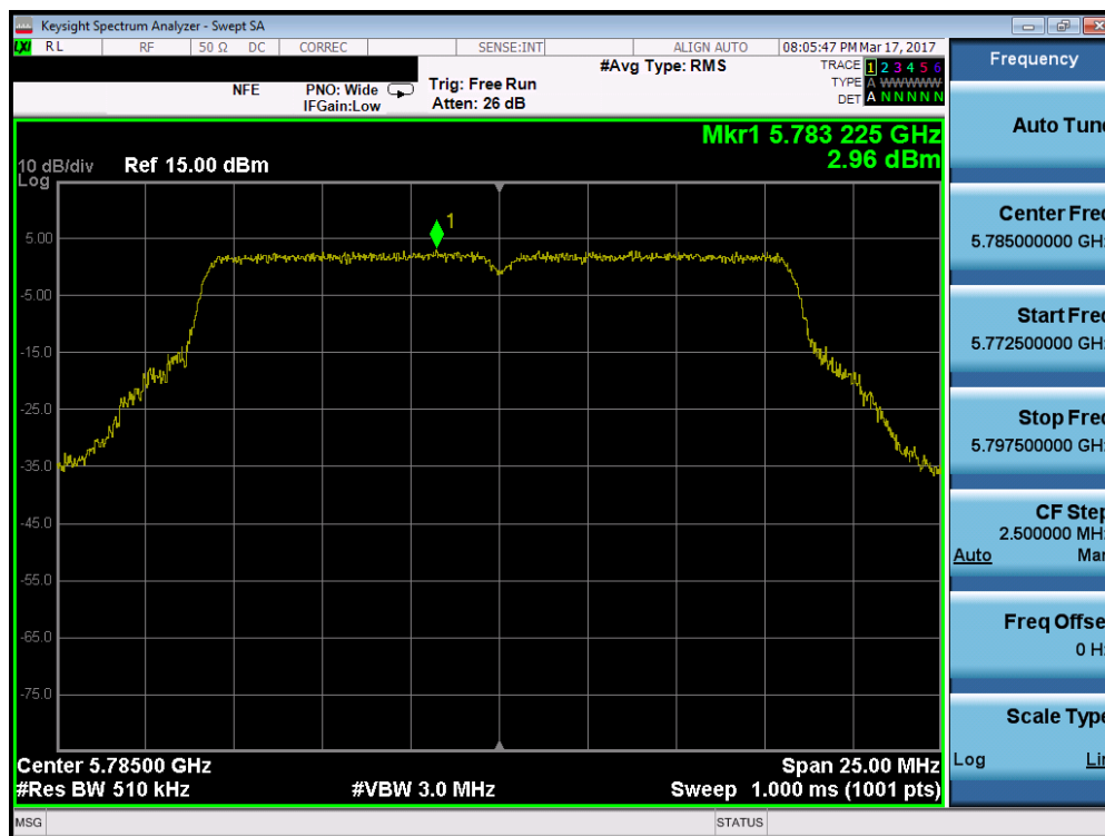
Plot 7-110. Power Spectral Density Plot (802.11a (UNII Band 3) - Ch. 157)
