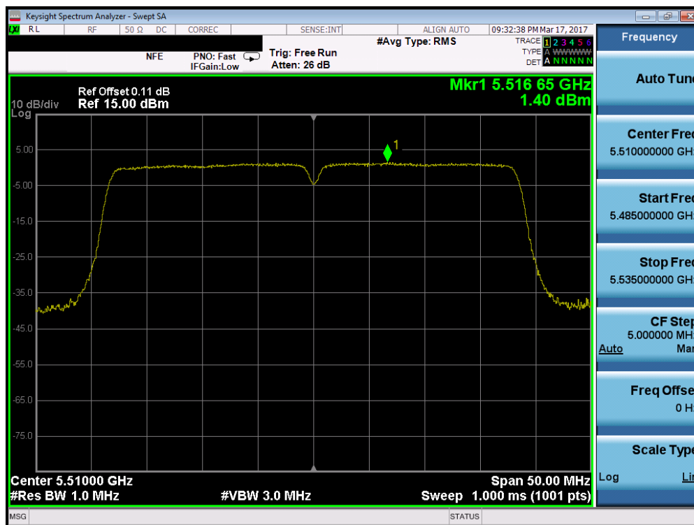
Plot 7-142. Power Spectral Density Plot (40MHz BW 802.11n (UNII Band 2C) – Ch. 102)
