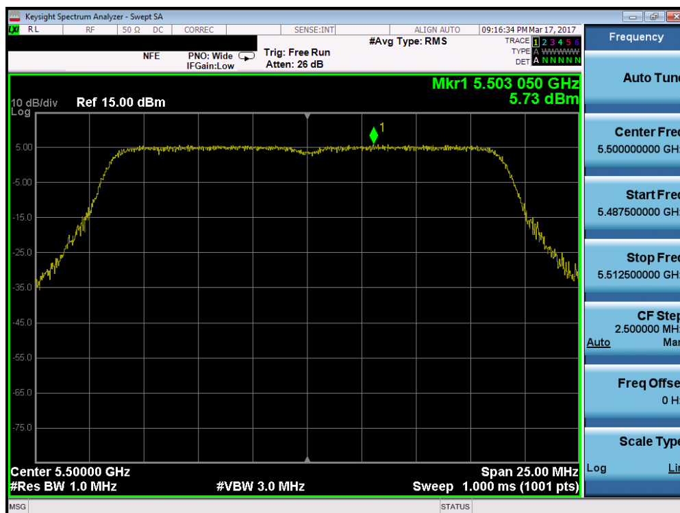
Plot 7-139. Power Spectral Density Plot (20MHz BW 802.11n (UNII Band 2C) – Ch. 100)
