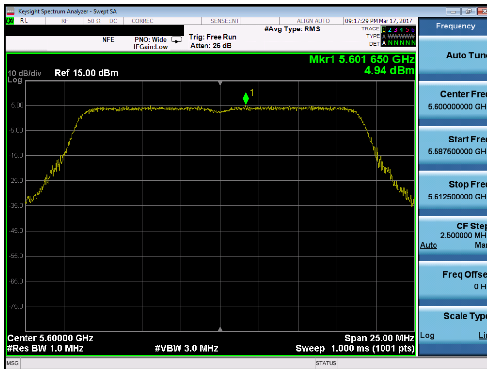
Plot 7-140. Power Spectral Density Plot (20MHz BW 802.11n (UNII Band 2C) – Ch. 120)
