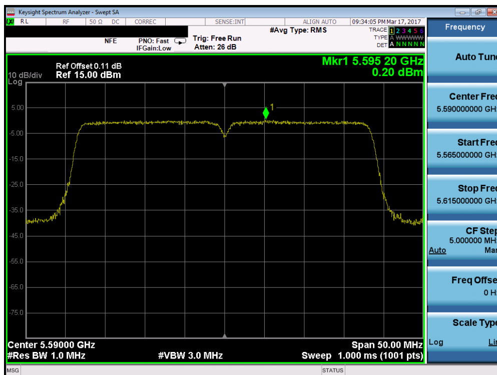
Plot 7-143. Power Spectral Density Plot (40MHz BW 802.11n (UNII Band 2C) – Ch. 118)
