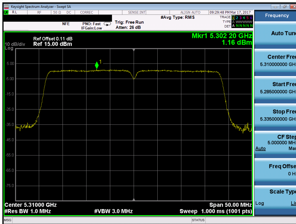
Plot 7-134. Power Spectral Density Plot (40MHz BW 802.11n (UNII Band 2A) – Ch. 62)
