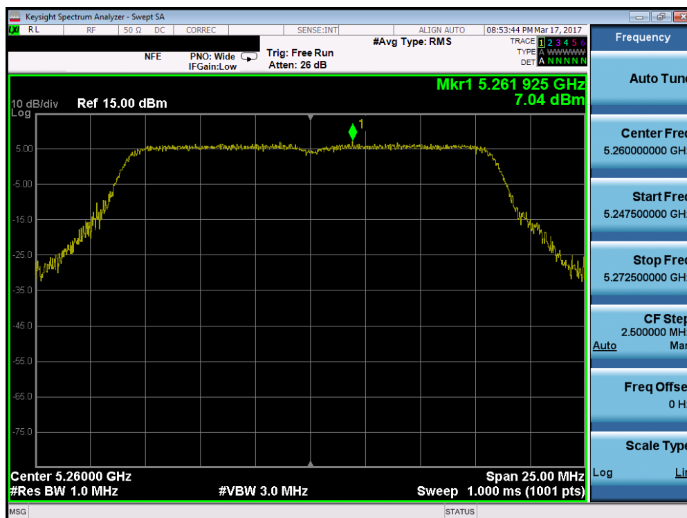
Plot 7-127. Power Spectral Density Plot (802.11a (UNII Band 2A) – Ch. 52)
