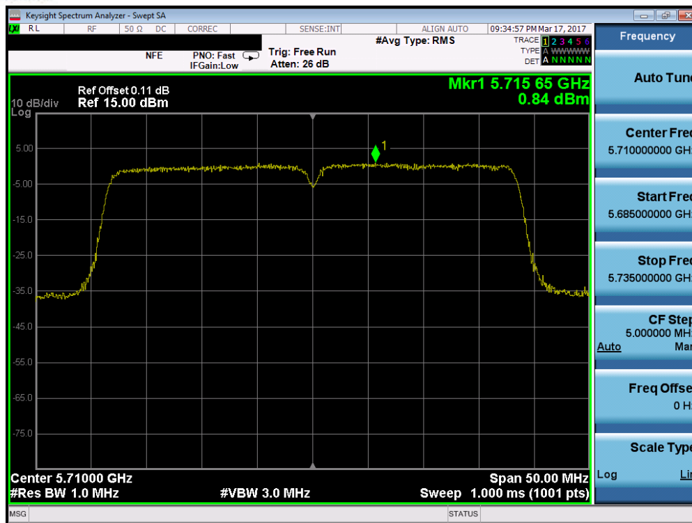
Plot 7-144. Power Spectral Density Plot (40MHz BW 802.11n (UNII Band 2C) – Ch. 142)
