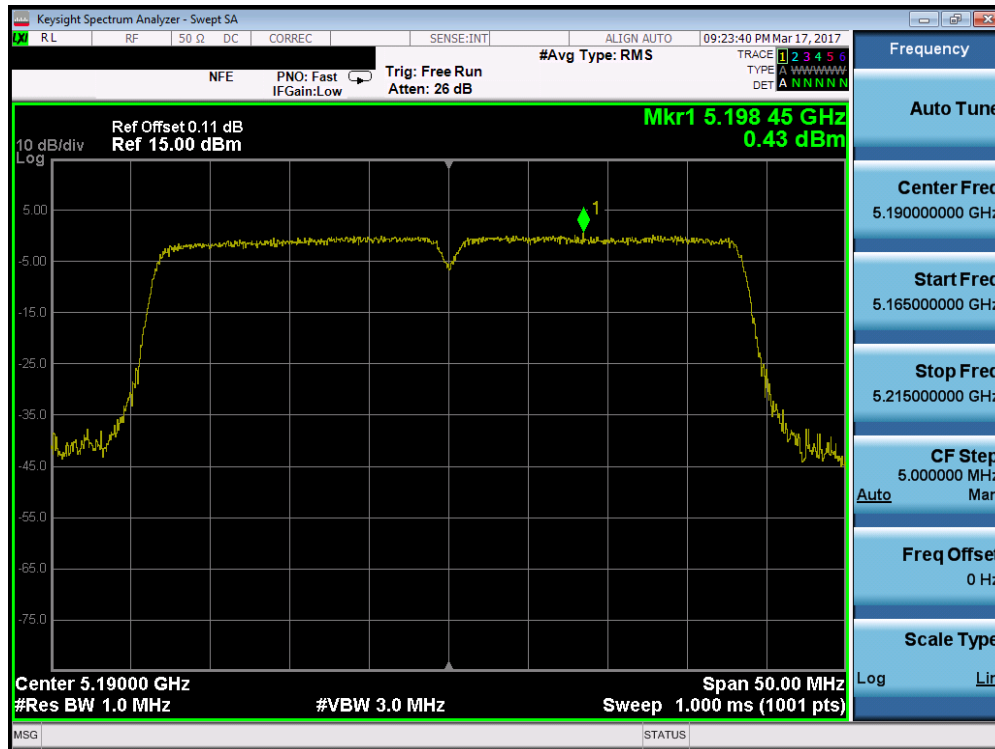
Plot 7-124. Power Spectral Density Plot (40MHz BW 802.11n (UNII Band 1) – Ch. 38)
