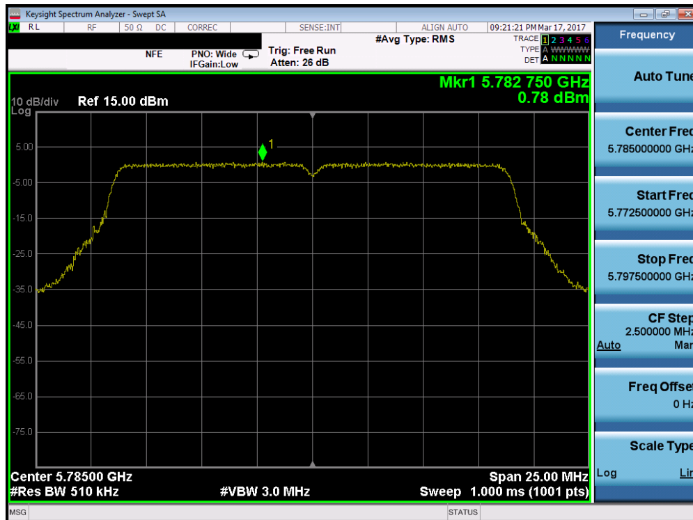
Plot 7-152. Power Spectral Density Plot (20MHz BW 802.11n (UNII Band 3) – Ch. 157)
