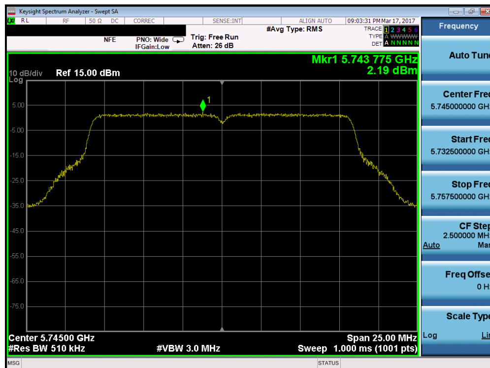
Plot 7-148. Power Spectral Density Plot (802.11a (UNII Band 3) – Ch. 149)
