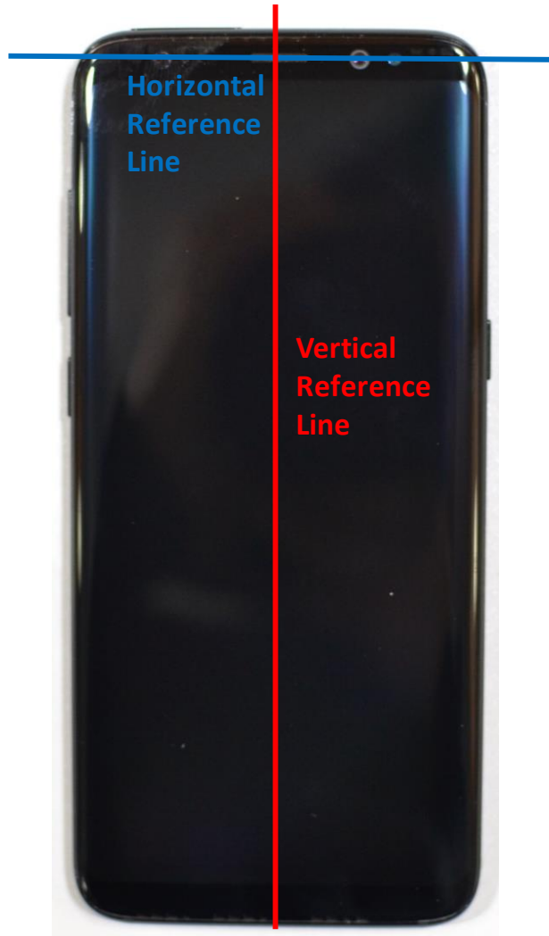
SAR Test Setup Photo 12 - Horizontal and Vertical Reference Lines
