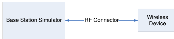
Figure 9-1 Power Measurement Setup
