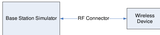
Figure 9-1 Power Measurement Setup
