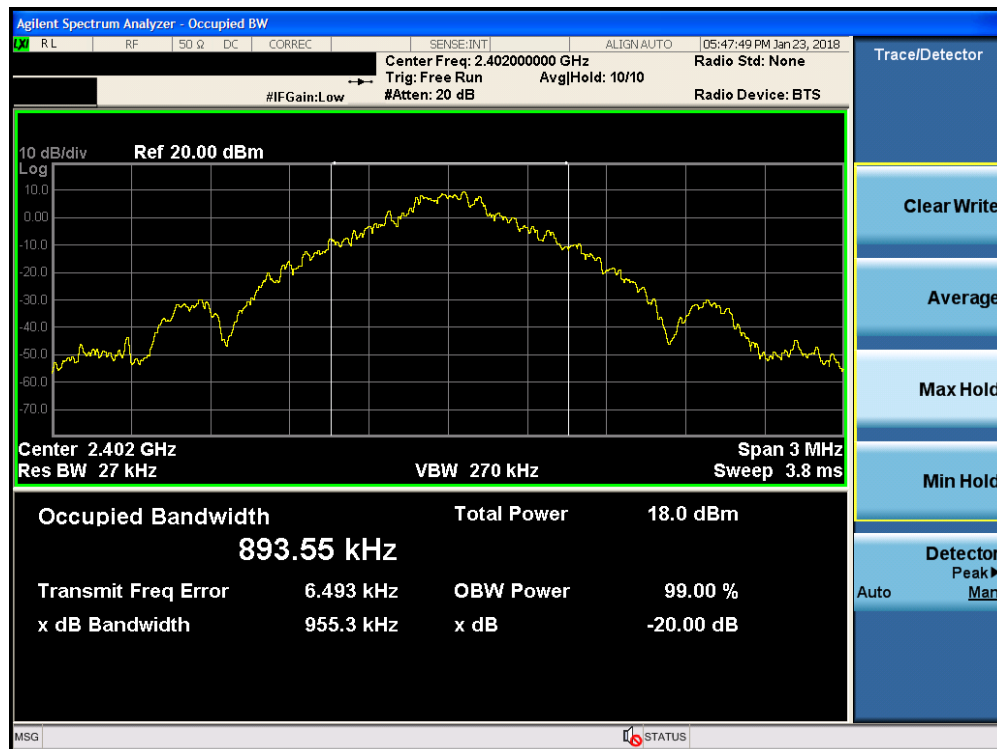
Plot 7-1. 20dB Bandwidth Plot (Bluetooth, 1Mbps – Ch. 0)
