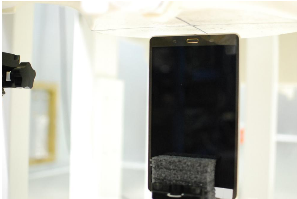
SAR Test Setup Photo 4: Bottom Edge at 1.1 cm
