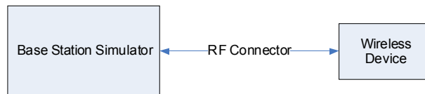
Figure 9-2 Power Measurement Setup
