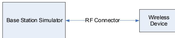
Figure 9-1 Power Measurement Setup
