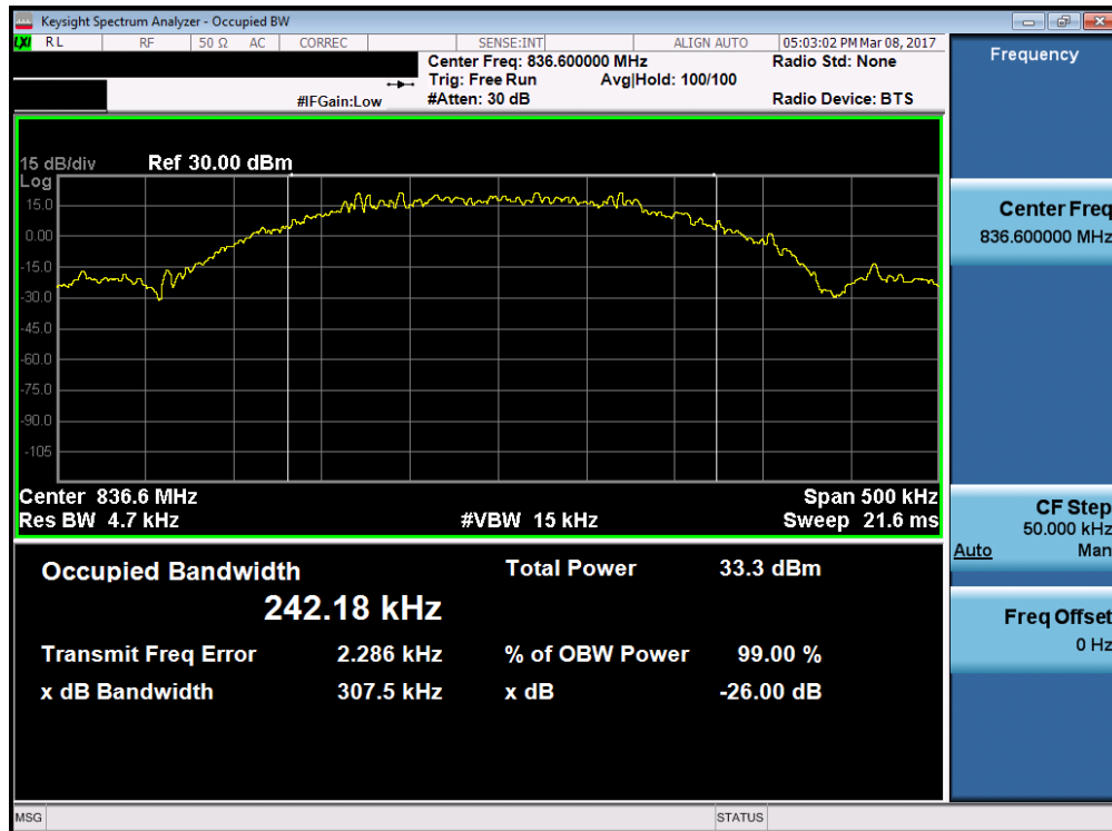
Plot 7-2. Occupied Bandwidth Plot (EDGE850 Mode – Ch. 190)
