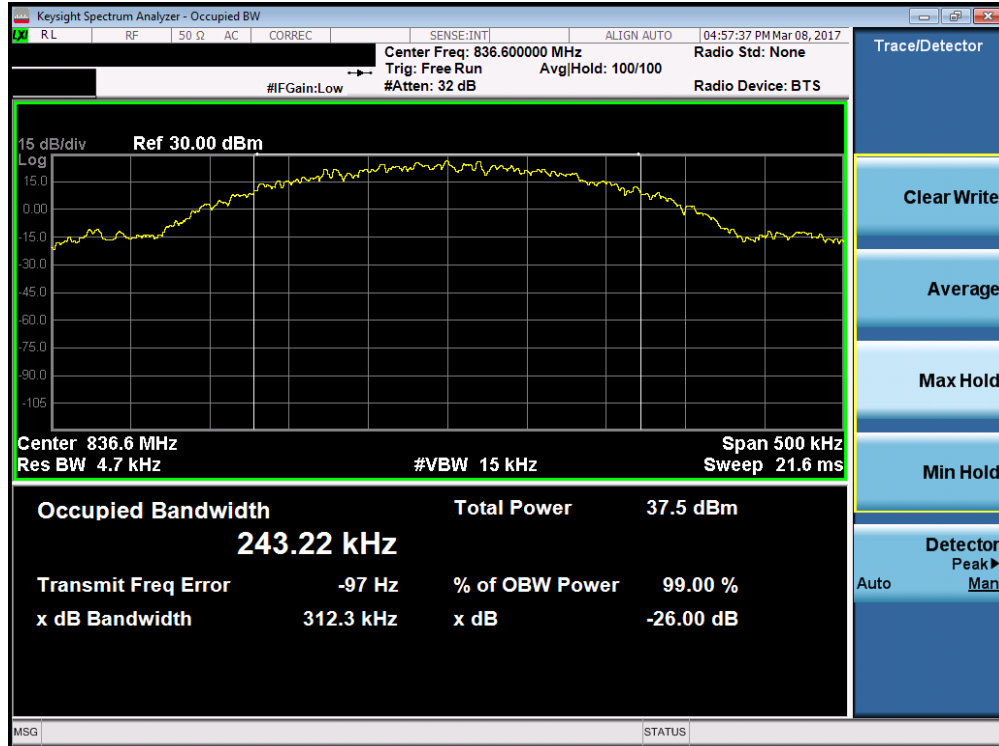
Plot 7-1. Occupied Bandwidth Plot (Cellular GSM Mode – Ch. 190)
