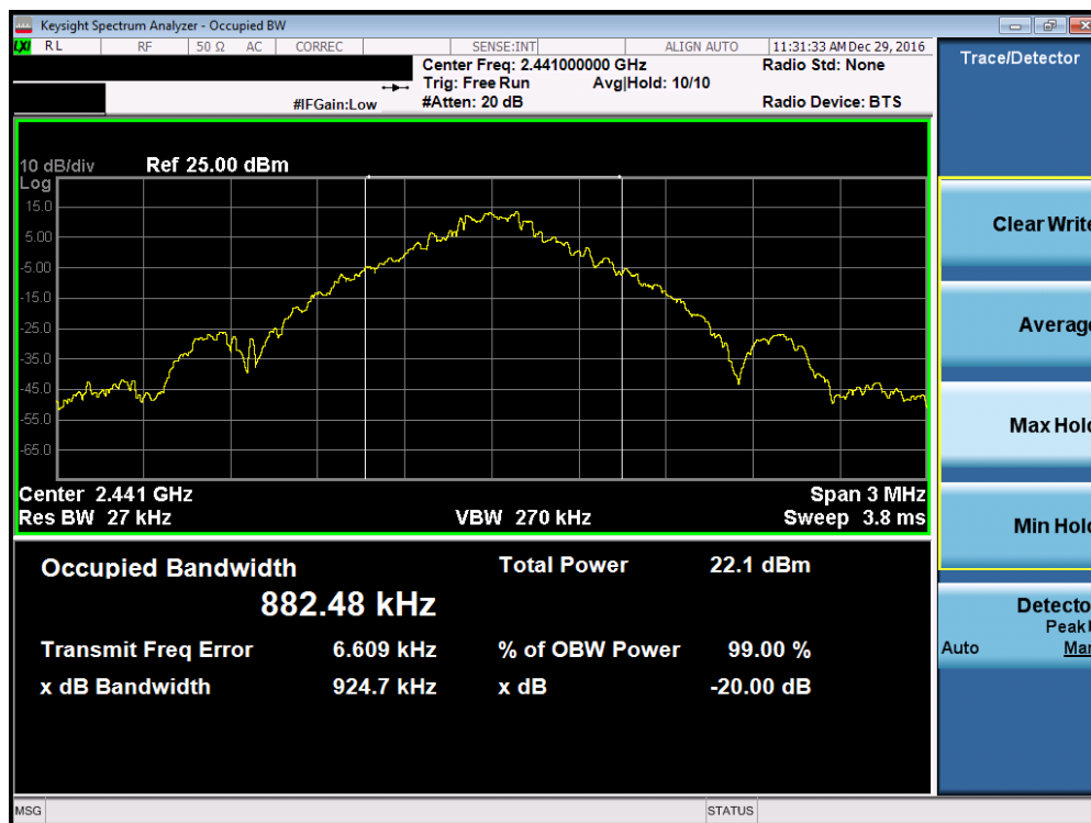
Plot 7-2. 20dB Bandwidth Plot (Bluetooth, 1Mbps – Ch. 39)
