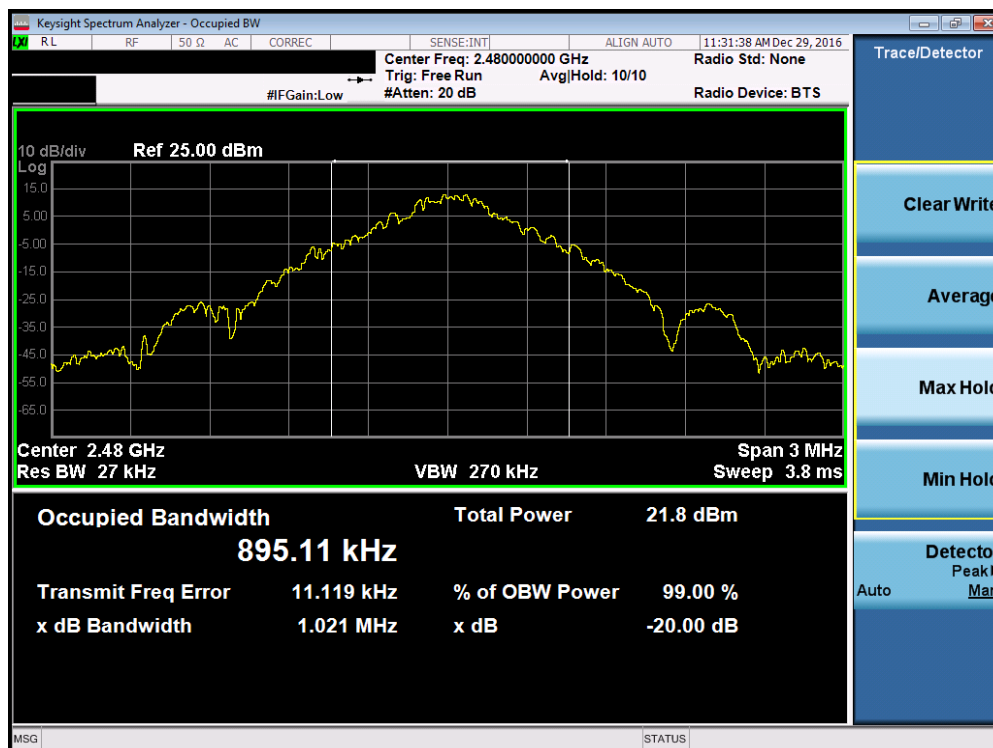
Plot 7-3. 20dB Bandwidth Plot (Bluetooth, 1Mbps – Ch. 78)
