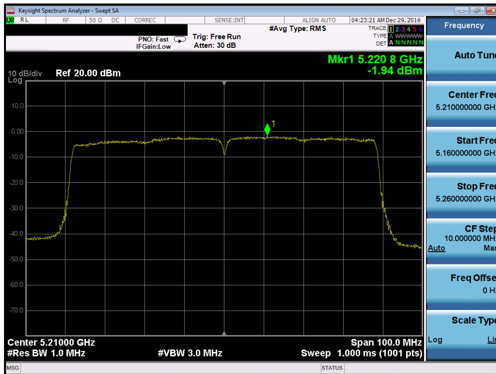
Plot 7-126. Power Spectral Density Plot (80MHz BW 802.11ac (UNII Band 1) – Ch. 42)
