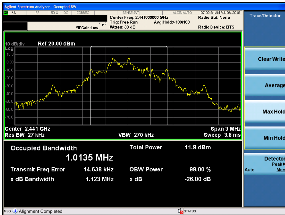
Plot 7-1. Occupied Bandwidth Plot (ANT+ – Ch. 39)
