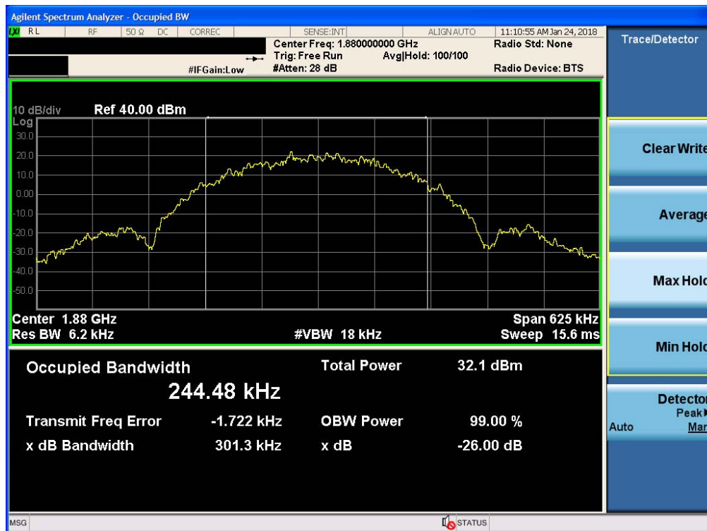
Plot 7-4. Occupied Bandwidth Plot (EDGE1900 Mode)
