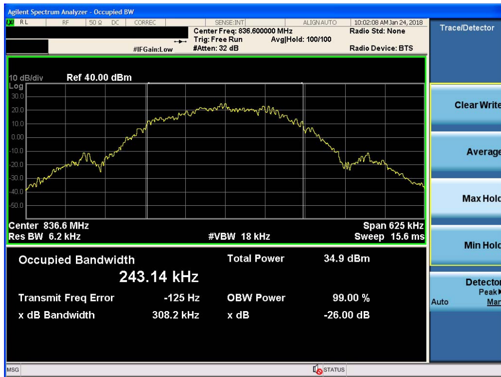
Plot 7-2. Occupied Bandwidth Plot (EDGE850 Mode)
