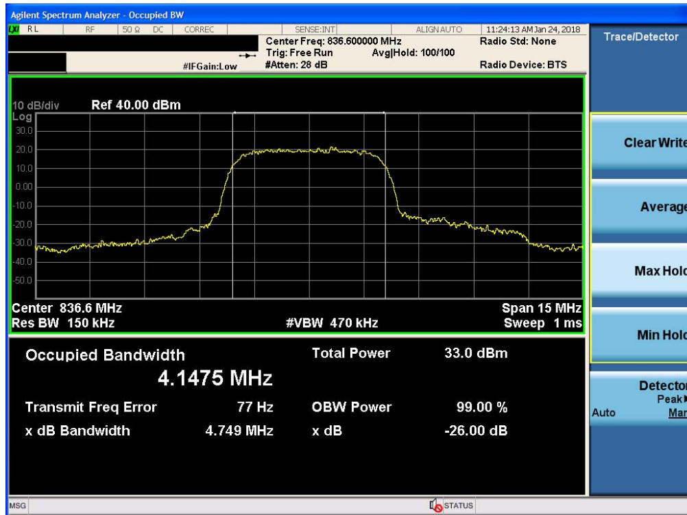
Plot 7-5. Occupied Bandwidth Plot (Cellular WCDMA Mode)
