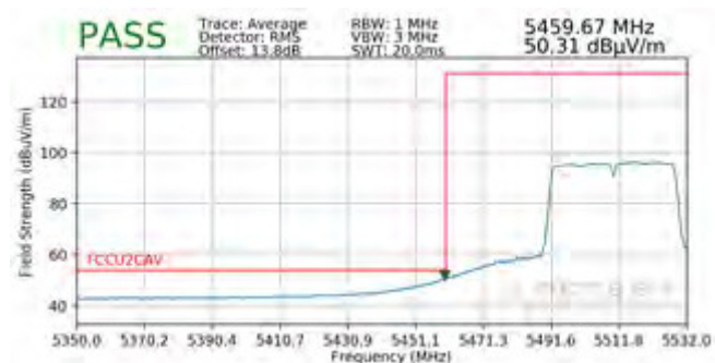
Plot 7-221. Radiated Band Edge Plot (Average – WCP)
