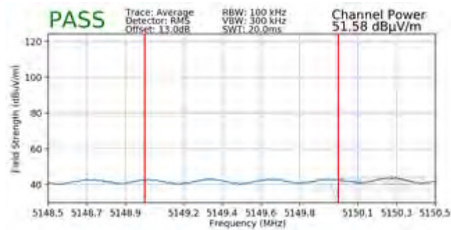
Plot 7-248. Radiated Band Edge Plot (Average – WCP)
