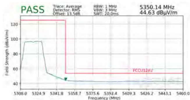
Plot 7-212. Radiated Band Edge Plot (Average – WCP)
