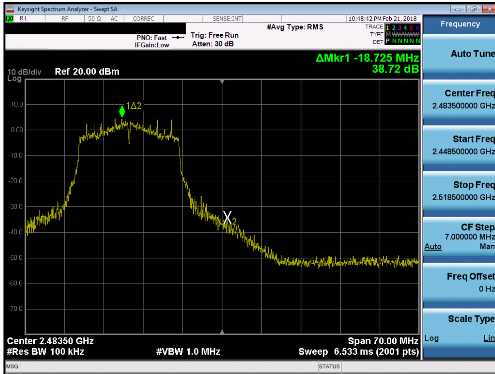
Plot 7-47. Band Edge Plot (802.11n (2.4GHz) – Ch. 12)
