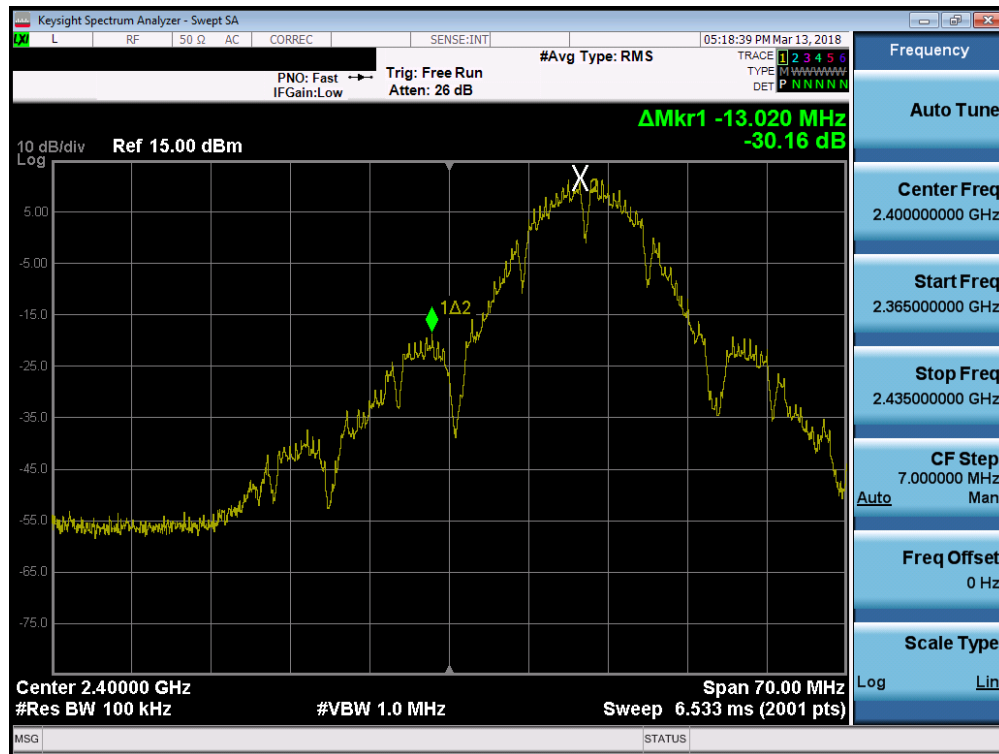
Plot 7-49. Band Edge Plot (802.11b – Ch. 1)
