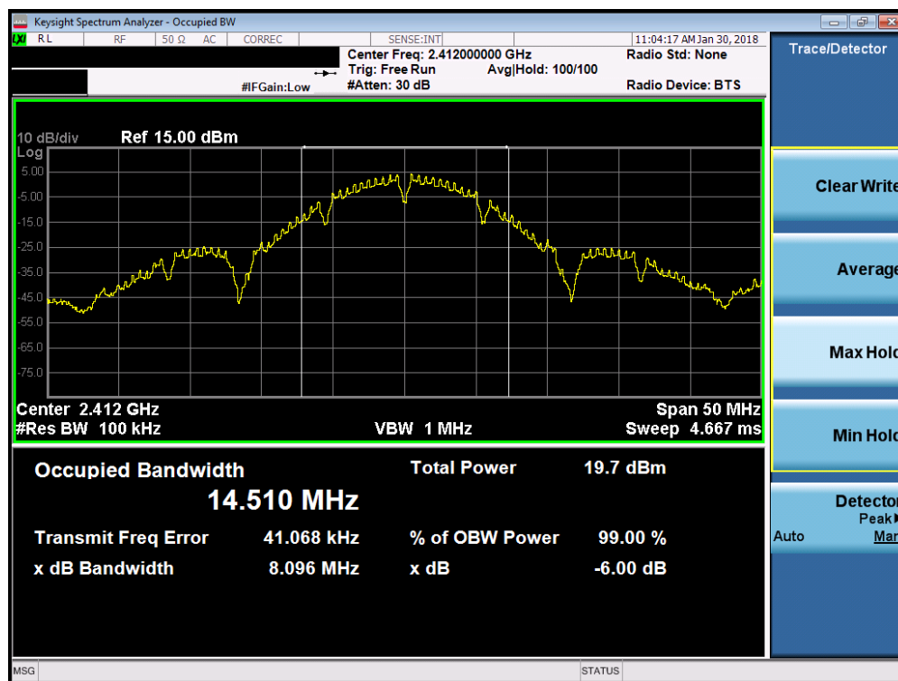
Plot 7-1. 6dB Bandwidth Plot (802.11b – Ch. 1)
