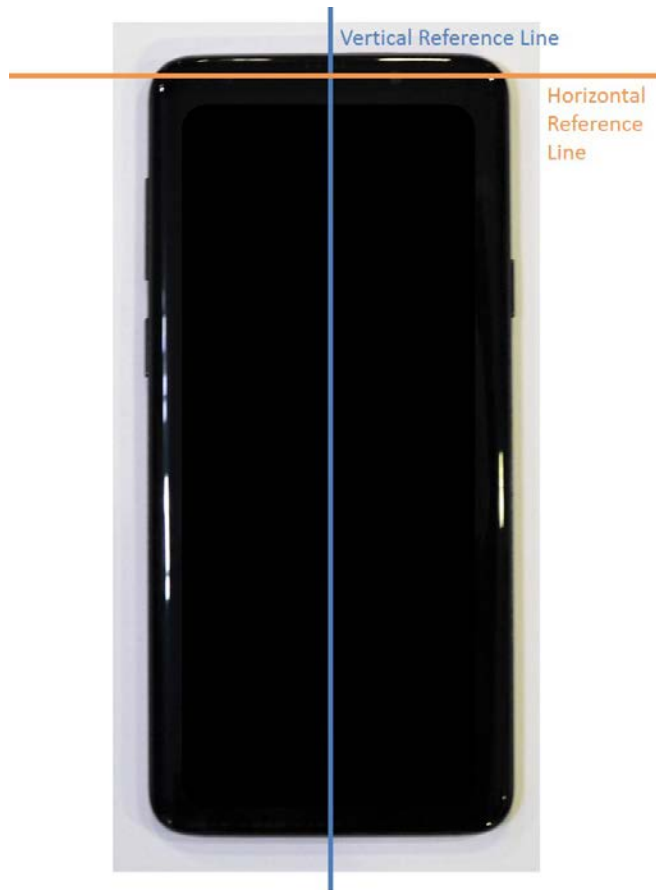
SAR Test Setup Photo 20 – Horizontal and Vertical Reference Lines
