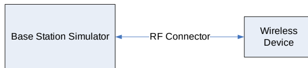
Figure 9-1 Power Measurement Setup
